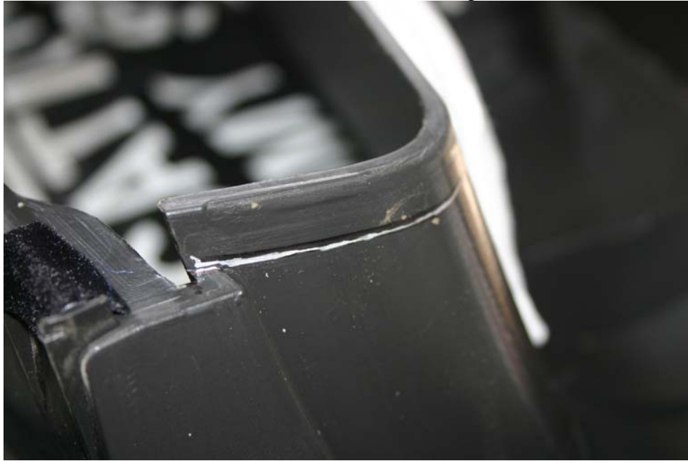
Upper panel back lower corner shown above – line indicates where cut should occur.
