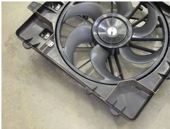
Fig. 3AC: Radiator Fan Shroud Air Dam Placement
