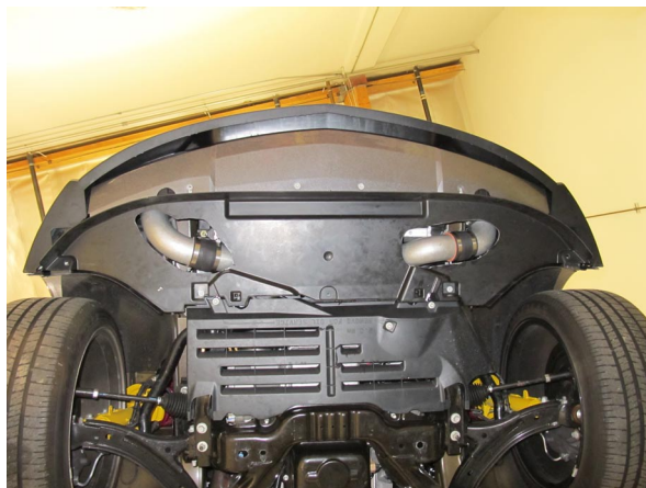
Fig. 12E-3: Plastic Undertray Trimming
