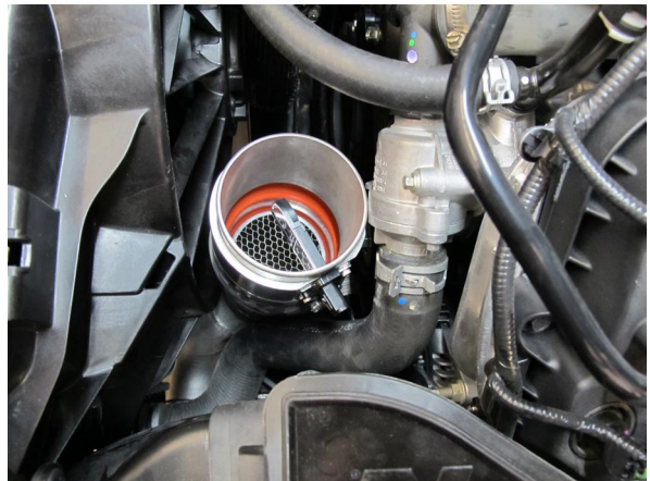
Fig. 7C-5: MAF Location (orientation will vary)
