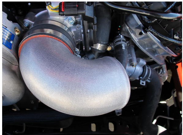
Fig. 7C-6: Ø3.5" x 120° Cast Aluminum Elbow
