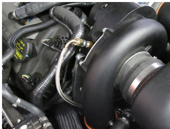
Fig. 13C: 90° Oil Feed Hose Installed
