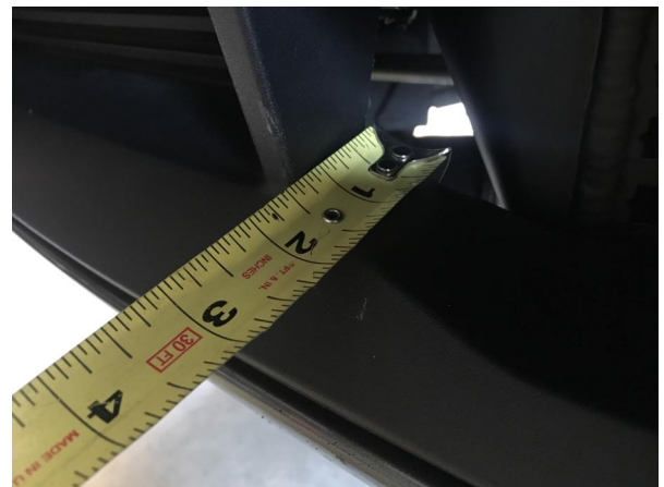
Fig. 12D-5: Bumper Cover, Center; Cut Line Reference
