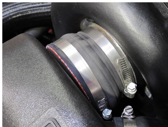
Fig. 11B: Air Inlet to Supercharger Connection
