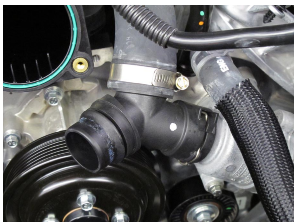
Fig. 2C: #28 Hose Clamp Orientation
