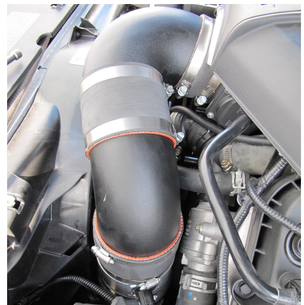
Fig. 7C-7: Cast Elbows, Final Position
