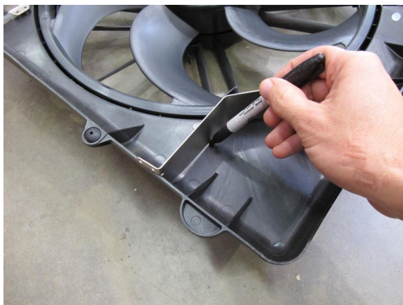
Fig. 3AD: Marking Air Dam Cut Lines
