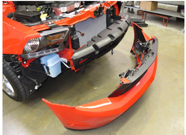
Fig. 1J: Front Fascia Removal
