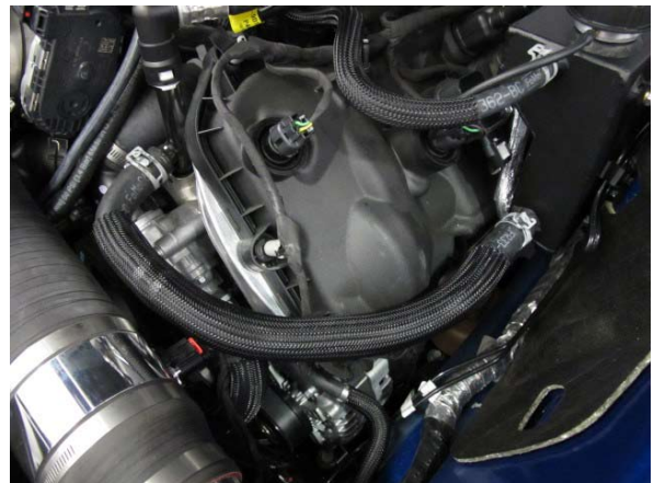
Fig. 3-w: Secure Modified OEM 3/4" Coolant Hose
