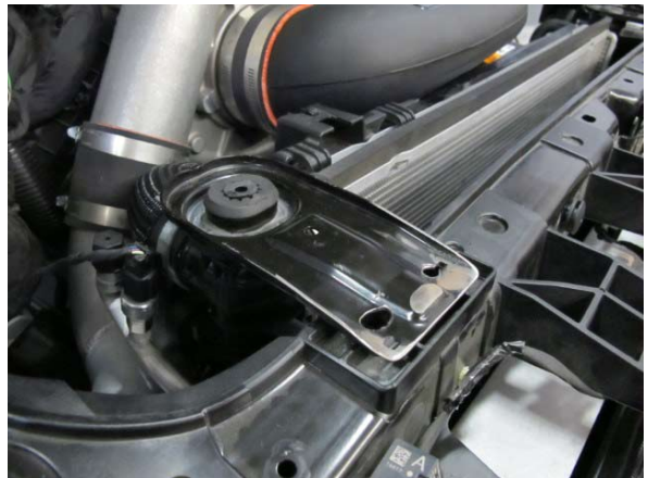
Fig. 3-g: Reinstall Modified Upper Radiator Brackets
