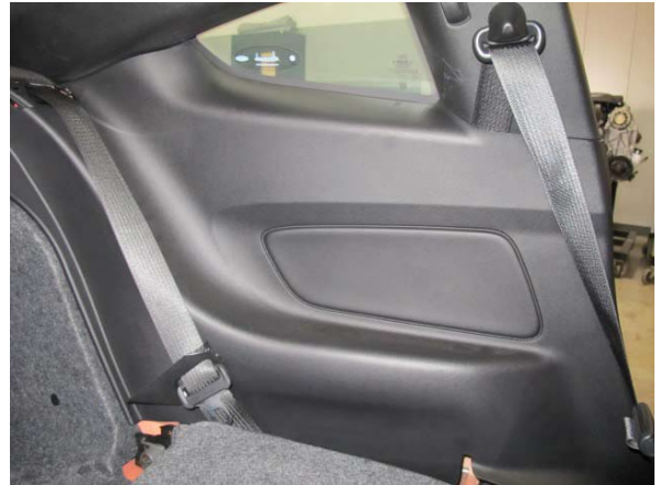
Fig. 6-p: Reinstall Driver Side Rear Interior Panel
