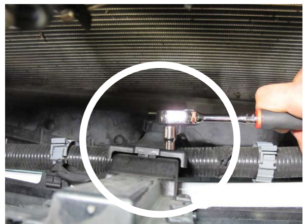
Fig. 1-r: Remove 2x 5mm-Headed Fasteners
