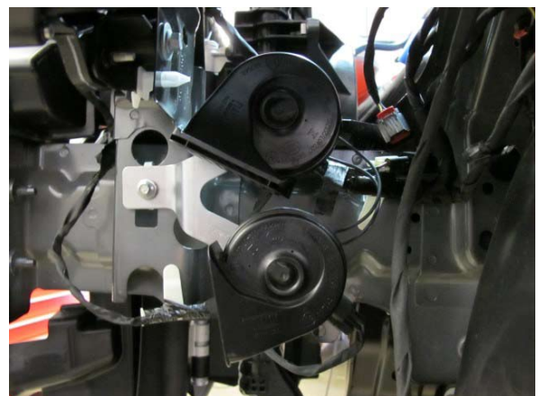
Fig. 4-ad: Remove Horn Assembly
