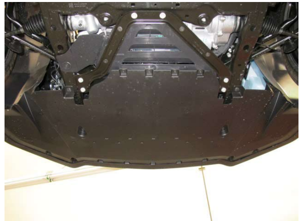
Fig. 1-k: Remove Lower Splash Guards
