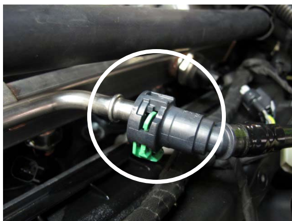
Fig. 5-f: Disconnect Low Pressure Fuel Feed Line
