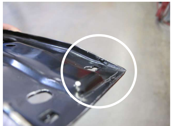
Fig. 3-f: Grind Down Raised Edges To A Taper
