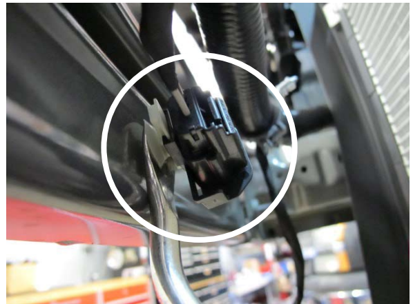
Fig. 4-n: Remove Unused Plug From Front Bumper Support
