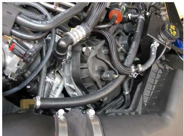
Fig. 7-i: Attach Breather Hose To Air Inlet
