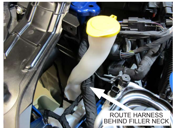
Fig. 4-k: Reinstall Windshield Washer Fluid Reservoir
