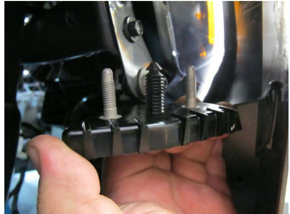
Fig. 1-j: Remove Corner Brackets
