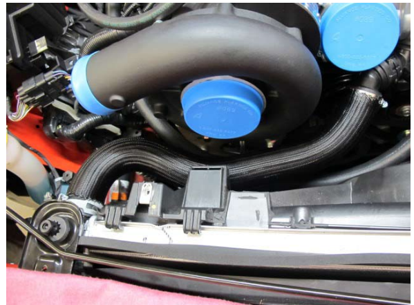
Fig. 3-k: Upper Radiator Hose (New Configuration)
