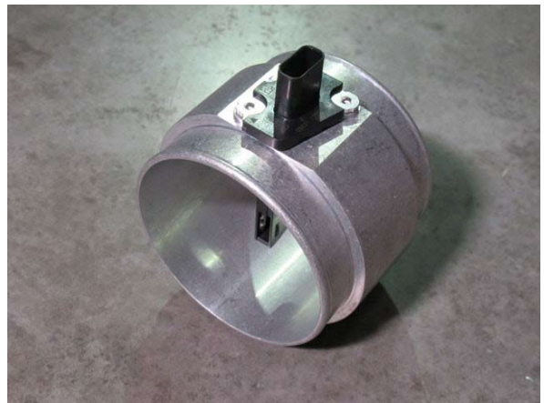
Fig. 4-ao: Install MAF Sensor To MAF Housing
