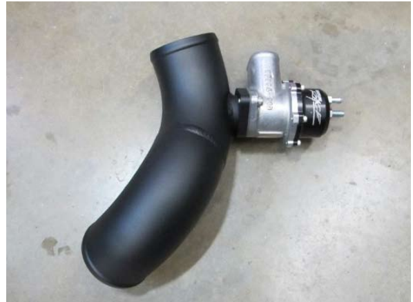
Fig. 4-ah: Install Bypass Valve (Automatic Transmission Vehicles)
