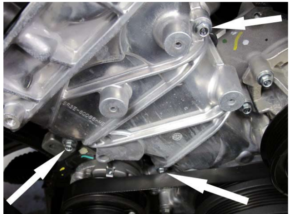
Fig. 2-a: Remove 3x Engine Cover Fasteners
