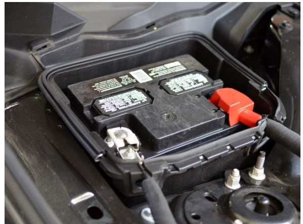
Fig. 1-b: Unplug Battery Leads
