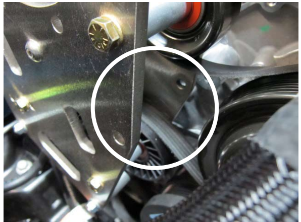
Fig. 2-n: Remove This 1x 2.730" Spacer & Set Aside
