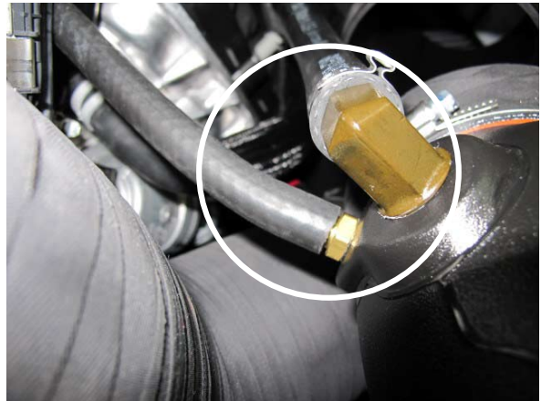
Fig. 7-m: Install 3/8" Hose, Then Secure Air Inlet Tube
