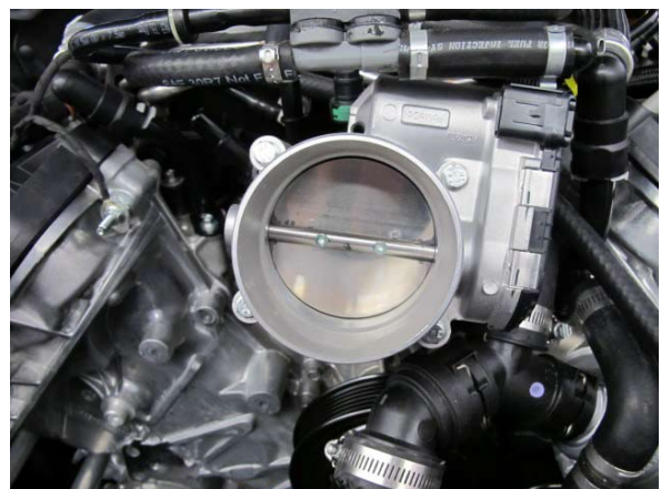
Fig. 4-c: Reinstall Throttle Body
