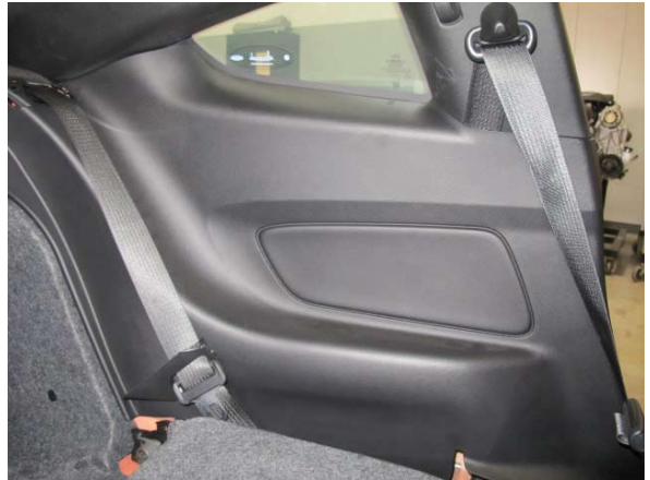
Fig. 6-g: Remove Driver Side Rear Interior Panel
