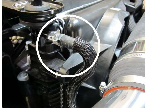
Fig. 3-m: Rotate The Driver Side OEM Molded Coolant Hose 90°
