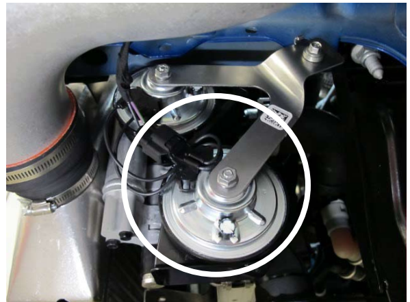
Fig. 4-au: Install Horn Assembly
