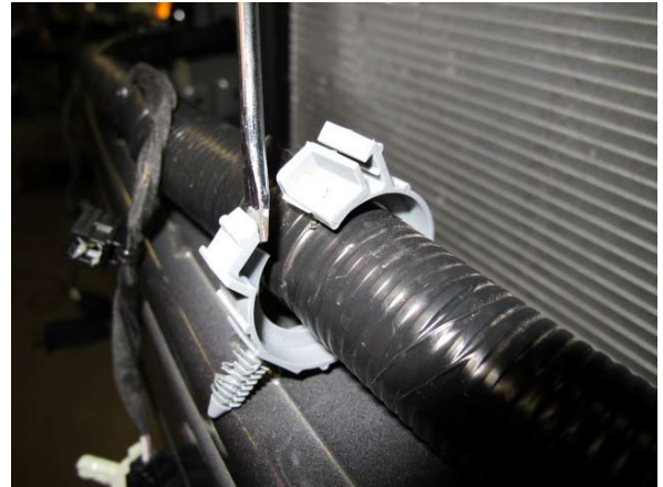
Fig. 4-p: Remove Gray Wire Harness Clips
