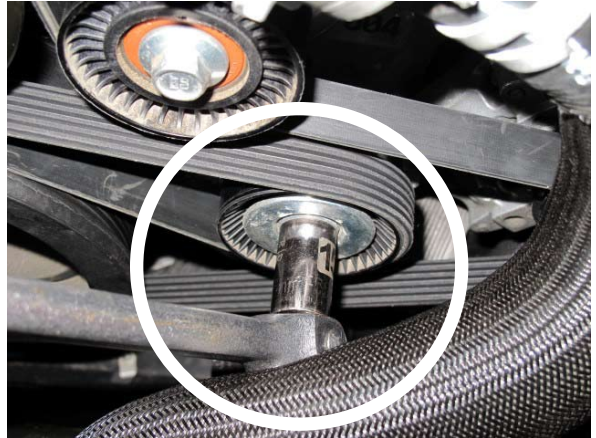
Fig. 2-s: Install Supercharger Drive Belt
