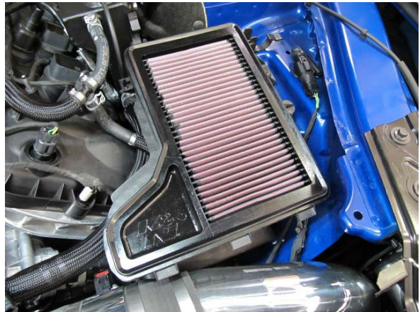
Fig. 7-h: Install Provided Air Filter & Secure OEM Air Box
