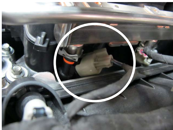
Fig. 5-d: Disconnect Fuel Injectors
