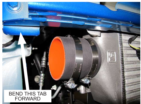
Fig. 4-aj: Install Silicone Sleeve & Hose Clamps
