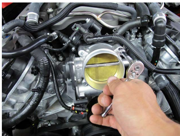
Fig. 1-aa: Remove Throttle Body
