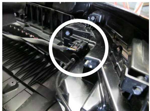
Fig. 1-l: Unplug Bumper Lights
