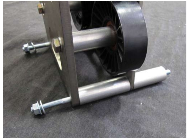
Fig. 2-h: Keep 2x 2.730" Spacers In Place
