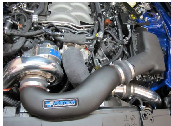
Fig. 7-l: Loosely Install Air Inlet Tube
