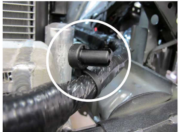
Fig. 4-q: Remove Plastic Harness Clip
