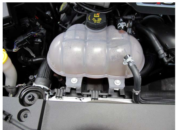
Fig. 1-x: Remove Coolant Reservoir
