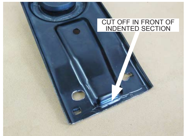
Fig. 3-e: Cut The Upper Radiator Bracket As Shown
