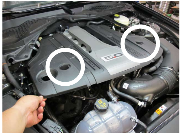
Fig. 1-t: Remove Engine Cover
