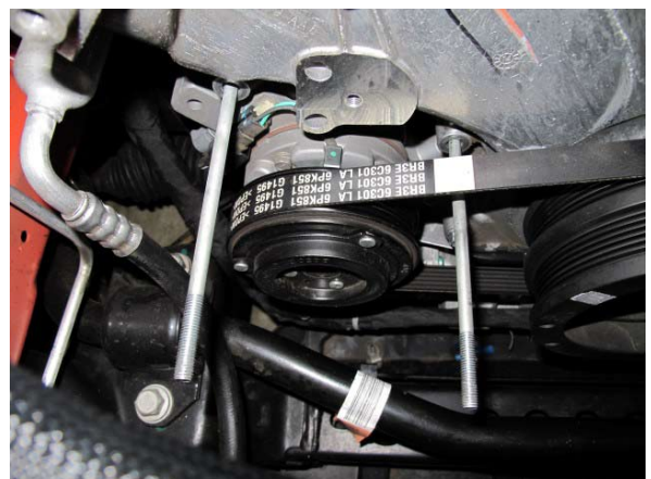
Fig. 2-f: Install Threaded Spacers
