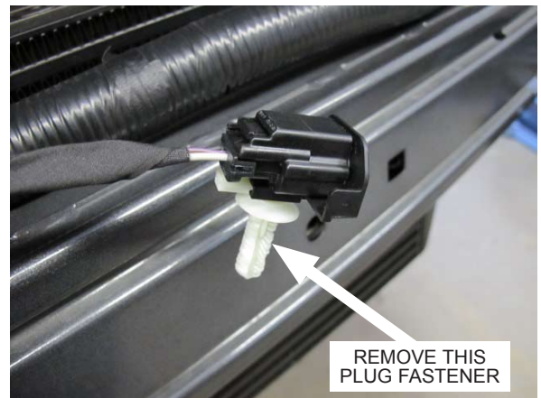
Fig. 4-z: Remove Plug Retainer
