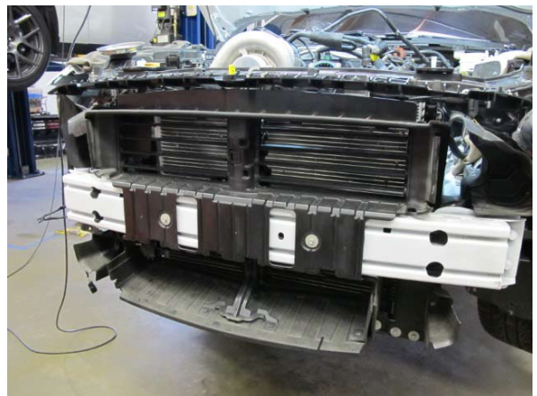
Fig. 1-o: Remove 8mm-Headed Fasteners
