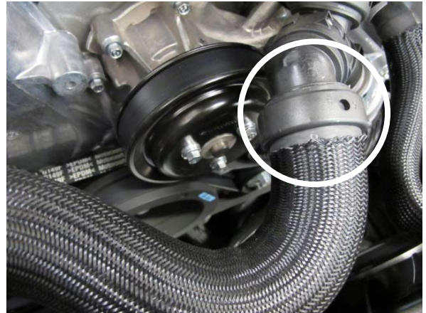
Fig. 3-j: Remove Plastic Hose Clamp
