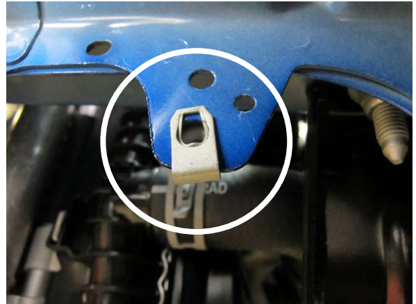
Fig. 4-at: Relocate OEM Threaded Clip
