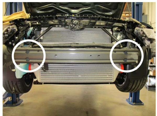
Fig. 4-x: Charge Air Cooler Installation
