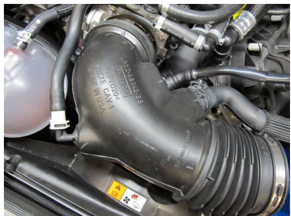
Fig. 1-u: Remove OEM Air Inlet
