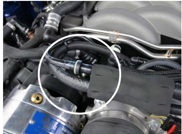
Fig. 7-k: Install 24" Length Of 3/8" Hose
