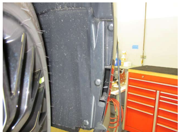
Fig. 1-f: Remove Fender Liner Fasteners
