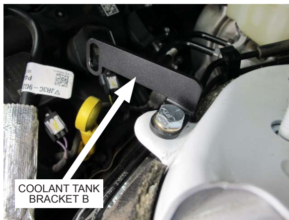
Fig. 3-q: Secure Coolant Tank Bracket B
