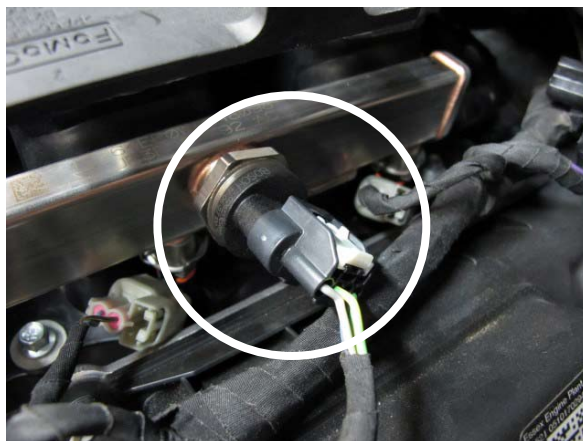
Fig. 5-e: Disconnect Fuel Rail Pressure Sensor
