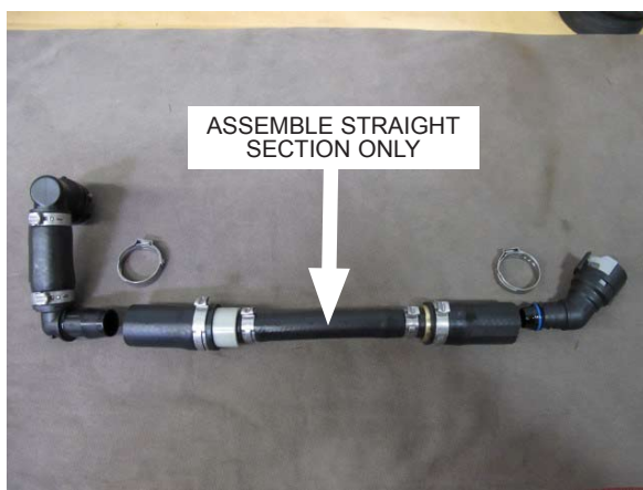
Fig. 7-c: Assemble Straight Section Of PCV Assembly
