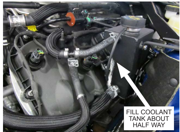
Fig. 3-y: Refill Cooling System
