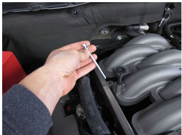
Fig. 5-o: Secure Fuel Rail Assembly
