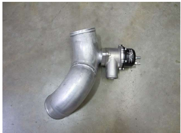
Fig. 4-ag: Install Bypass Valve (Manual Transmission Vehicles)
