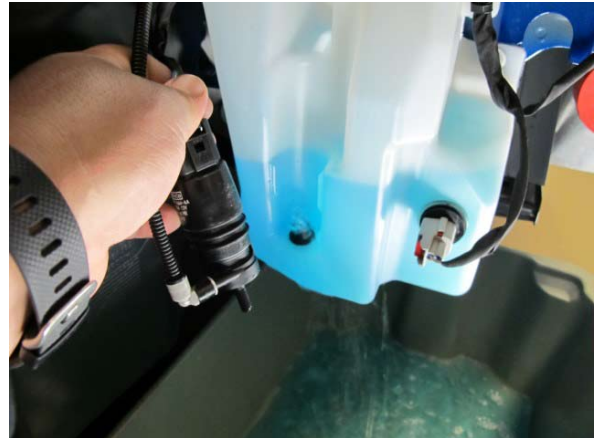
Fig. 4-d: Drain Windshield Washer Fluid Reservoir
