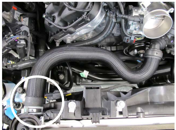
Fig. 3-i: Upper Radiator Hose (OEM Configuration)
