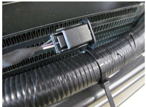
Fig. 4-aa: Secure Plug To Harness
