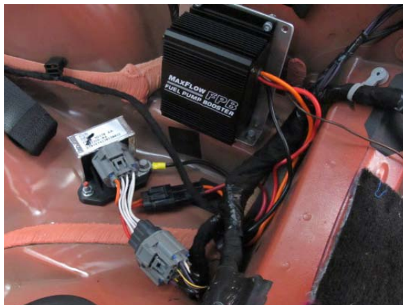
Fig. 6-m: Install Adapter Harness
