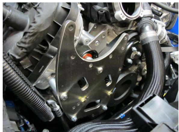
Fig. 2-i: Install Supercharger Mounting Bracket Assembly
