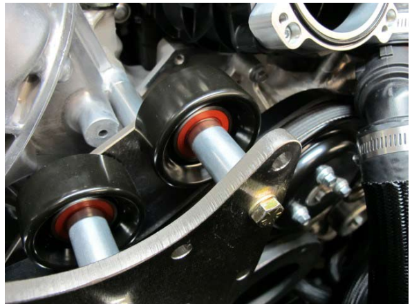
Fig. 2-m: Install Previously Removed Smooth Idler Pulley
