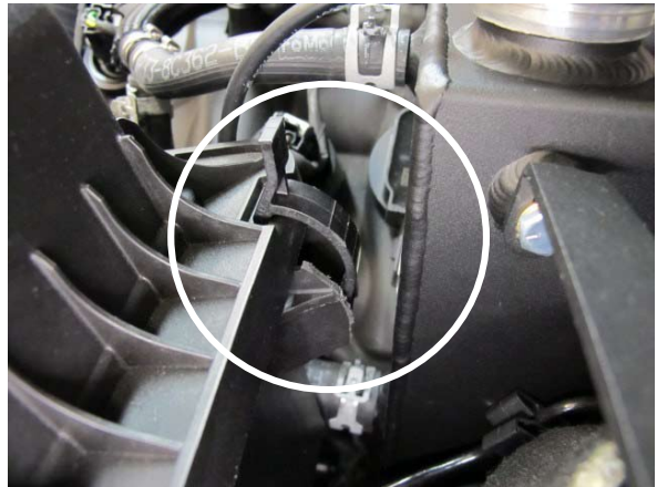
Fig. 7-g: Trim Air Box As Necessary
