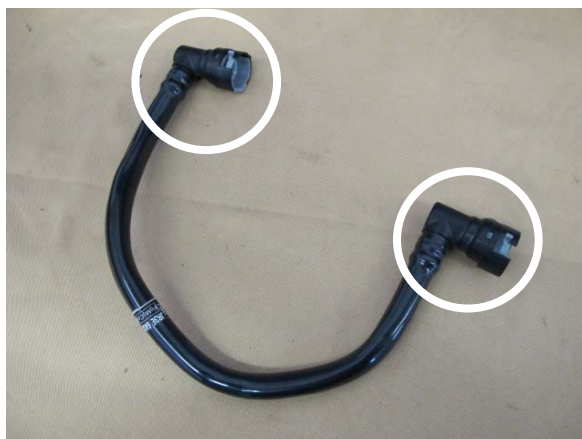
Fig. 7-a: Remove Both Quick-Release Fittings
