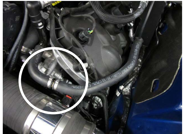
Fig. 3-v: OEM 3/4" Coolant Hose (Modified)
