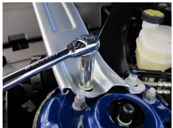
Fig. 1-c: Remove Strut Tower Brace
