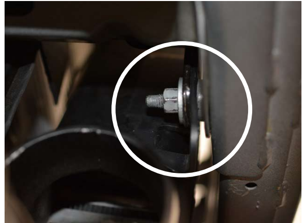
Fig. 4-y: Secure Charge Air Cooler
