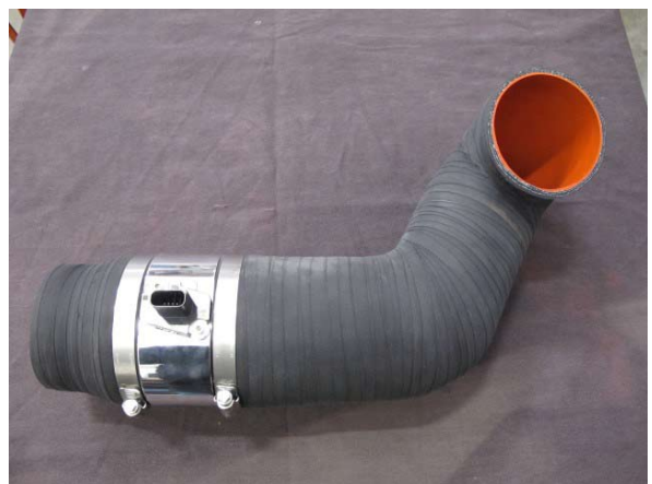
Fig. 4-ap: Assemble MAF Sensor Housing & Sleeves As Shown
