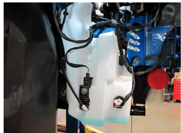
Fig. 4-l: Reinstall Windshield Washer Fluid Pump & Windshield Washer Fluid Level Sensor
