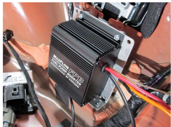
Fig. 6-l: Mount Fuel Pump Booster
