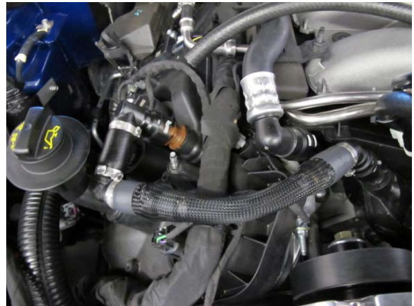
Fig. 7-e: Install PCV Assembly
