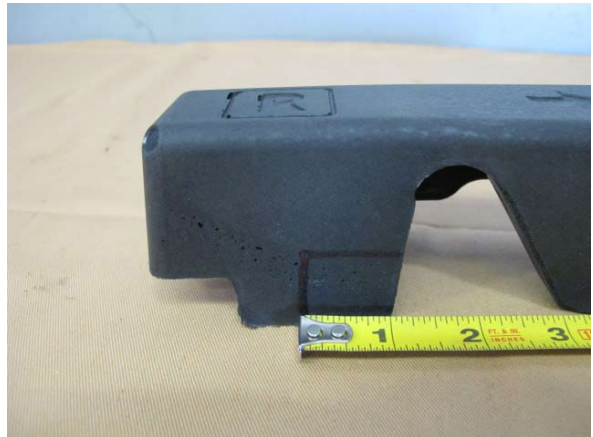
Fig. 5-m: Modify Passenger Side Fuel Rail Cover
