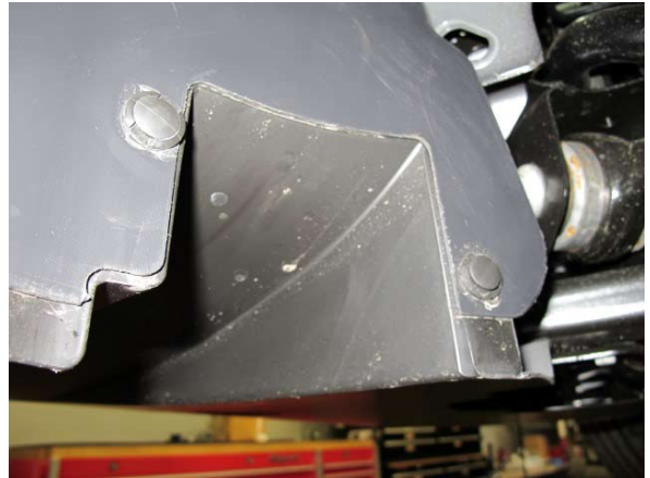
Fig. 1-g: Remove Plastic Fasteners
