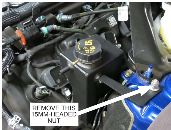
Fig. 3-r: Loosely Attach Coolant Tank
