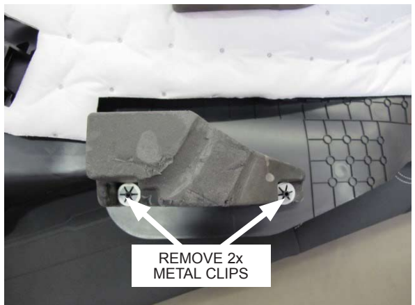
Fig. 6-i: Remove Foam Insulation Block
