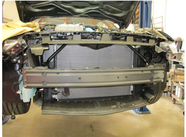
Fig. 1-m: Remove Front Bumper Cover
