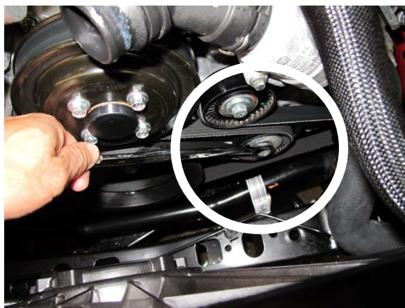
Fig. 1-z: Remove Accessory Drive Belt
