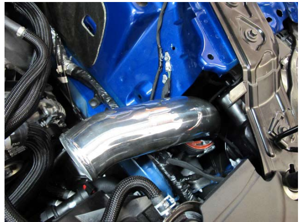
Fig. 4-an: Install Discharge Tube D
