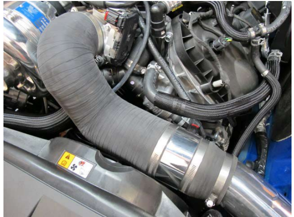
Fig. 4-aq: Secure All Hose Clamps
