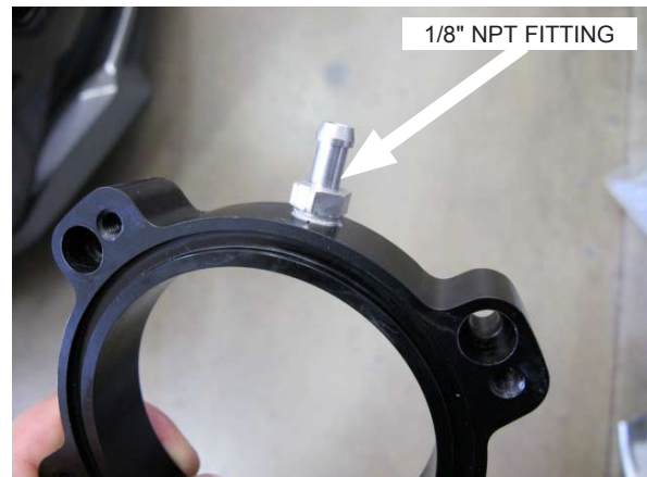
Fig. 4-a: Install 1/8" NPT Fitting
