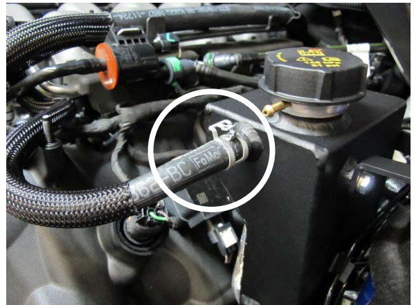
Fig. 3-t: Attach Upper OEM Molded Coolant Hose
