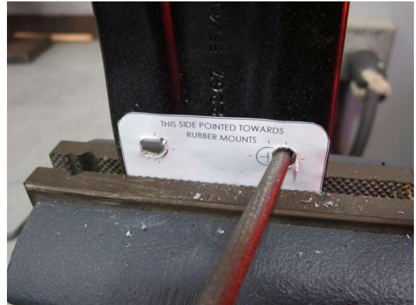
Fig. 3-d: Use Round File To Slot Hole
