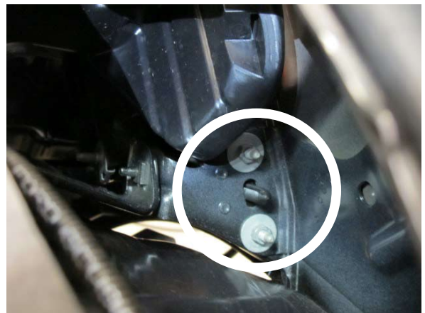
Fig. 1-i: Remove Corner Bracket Fasteners
