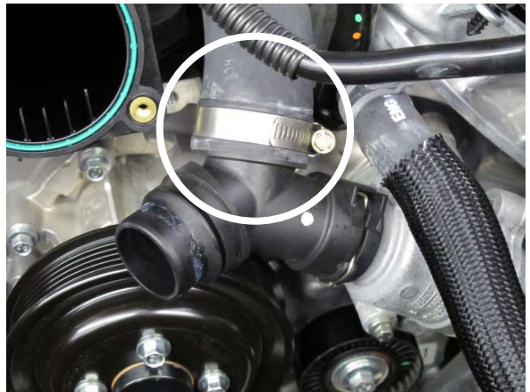
Fig. 3-h: Install #24 Hose Clamp
