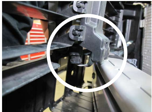
Fig. 1-s: Unplug Motor & Remove Active Grille Shutter Assembly
