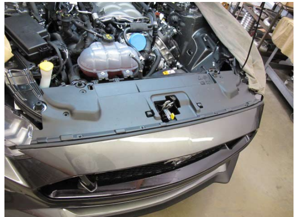
Fig. 1-d: Remove Radiator Support Cover
