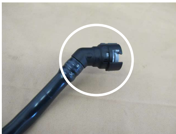
Fig. 7-b: Remove 45° Quick-Release Fitting
