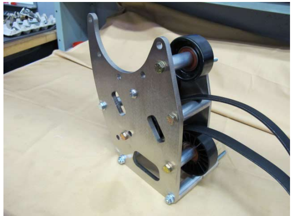
Fig. 2-b: Inspect Supercharger Mounting Bracket Assembly
