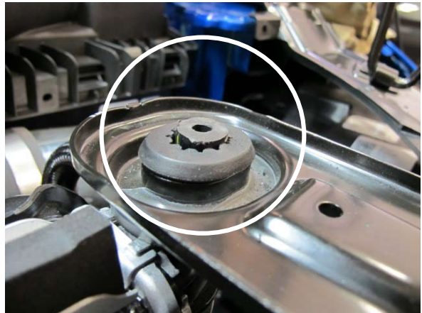
Fig. 7-n: Modify Radiator Mounting Tabs
