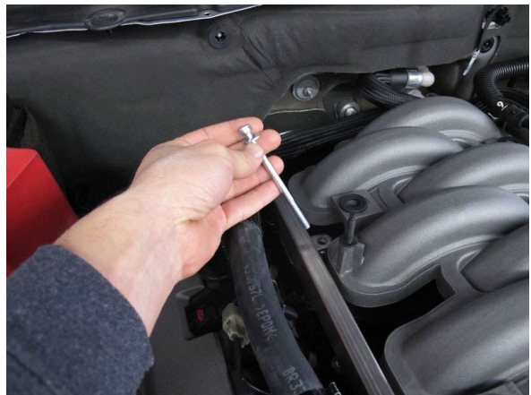
Fig. 5-h: Remove Fuel Rail Assembly
