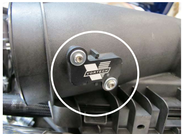
Fig. 7-f: Install MAF Block-Off Plate
