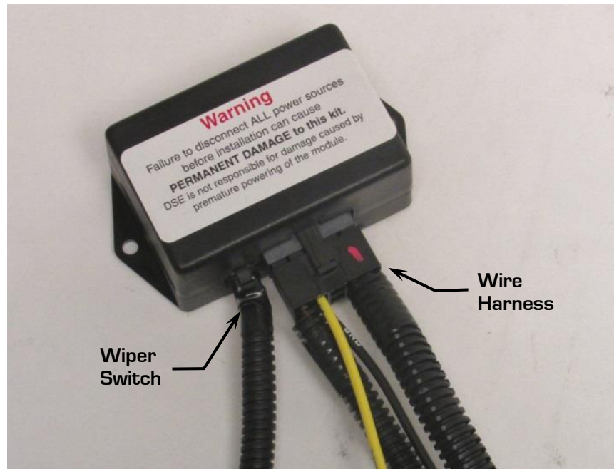
Figure 26– Connect Wiper Switch & Harness to Module
