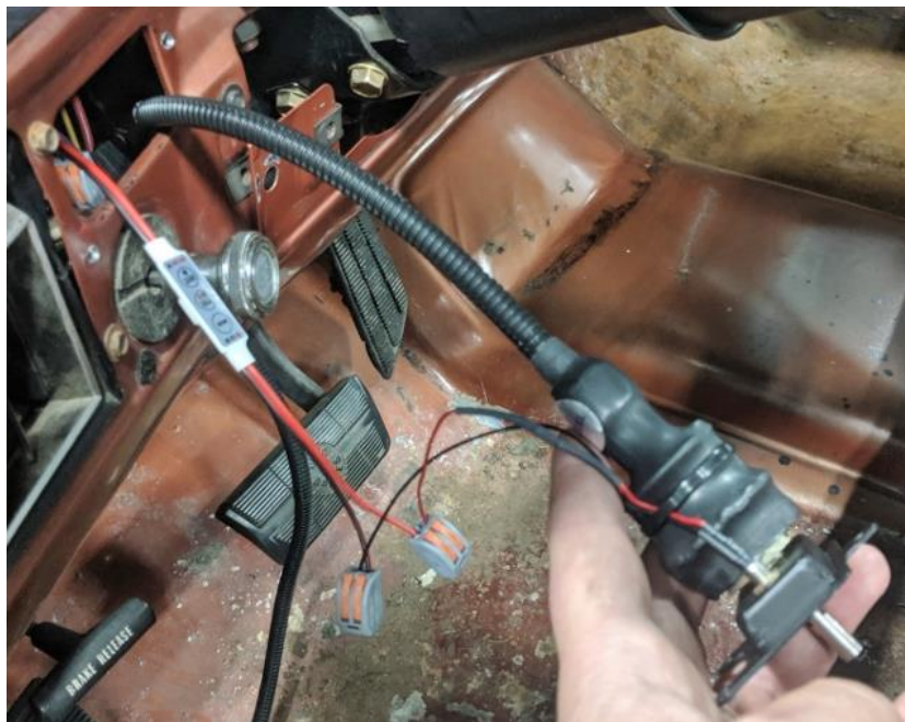
Figure 14 – Connect LED to Dimmer
