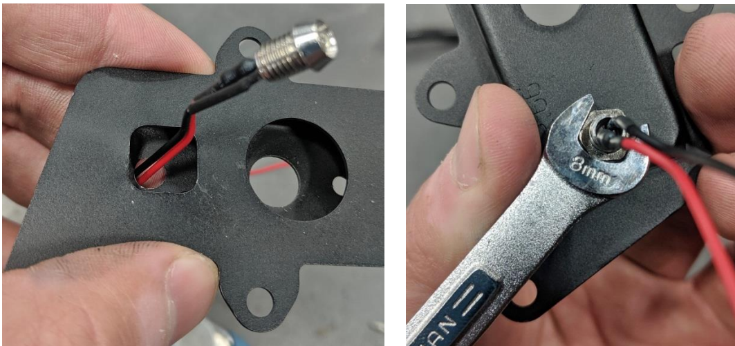
Figure 9 – Install LED into Light Box Assembly
