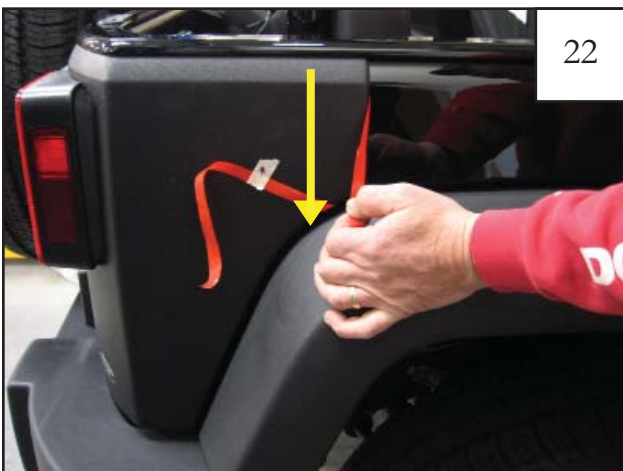
Pull tape liner 9 downward. NOTE: Refer to steps 8 & 9 for tape liner tab numbering.
