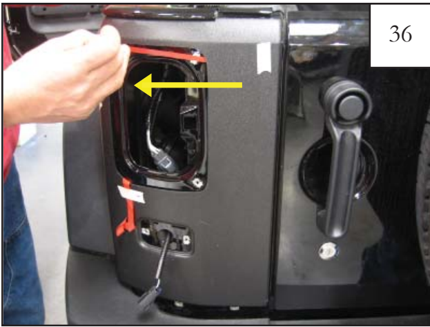
36 Pull tape liner 9 for the 1/4" tape to the left toward the driver side of the vehicle. NOTE: Refer to step 24 for tape liner tab numbering.
