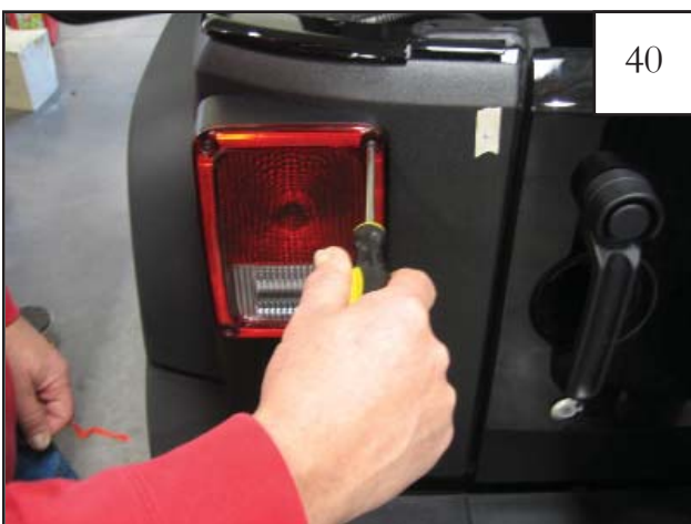
40 Using a #2 Phillips screwdriver, reinstall tail light.
