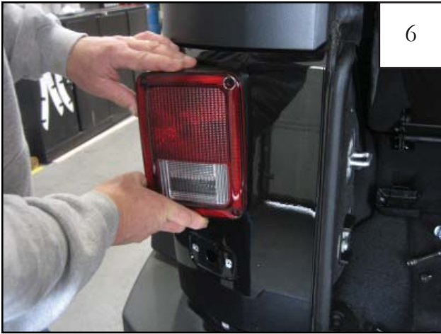
Slide light toward the inside of the vehicle then pull out to remove the tail light.
