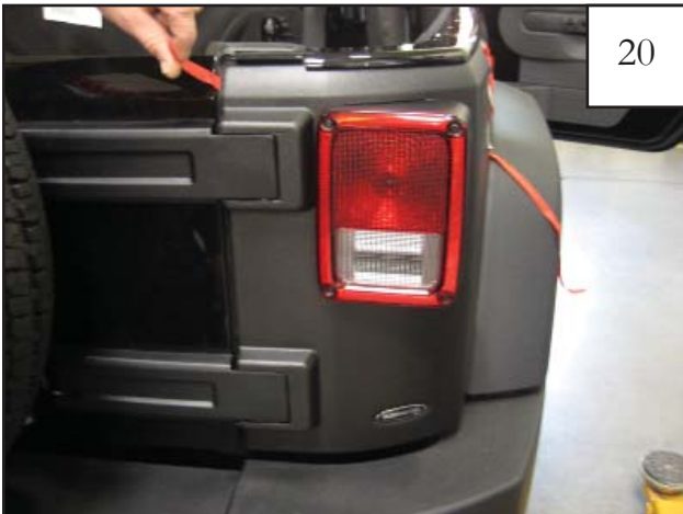
Press down on the part along the length where tape strip 7 is.
