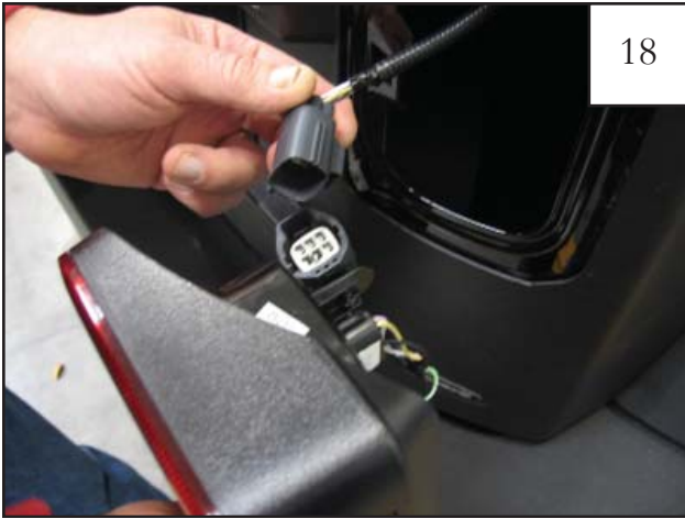
Plug the light connector back into the tail light and reinstall tail light using a #2 Phillips screwdriver.
