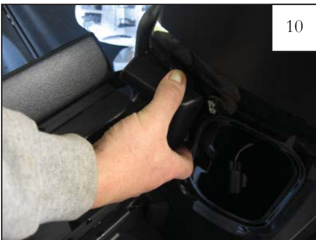
Slide covers off door hinges.
