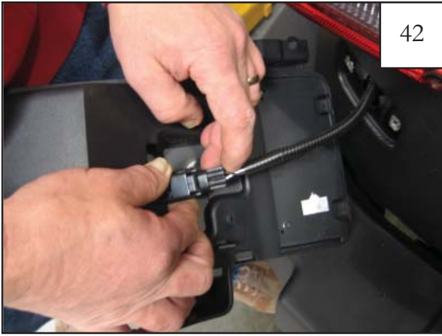
Reconnect light of license plate frame.
