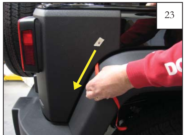
Pull tape liner 10 downward on a slight diagonal matching the curvature of the part. NOTE: Refer to steps 8 & 9 for tape liner tab numbering. Once all tape liners are peeled, press down on entire part again applying 30 PSI to the taped areas. NOTE: The tape reaches maximum adhesive bond after 24 hours of contact. Do not wash vehicle for 24 hours.
