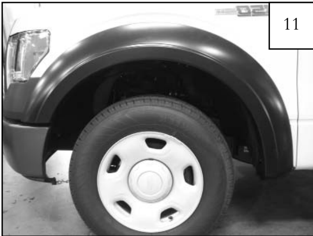
Completed front flare installation.
