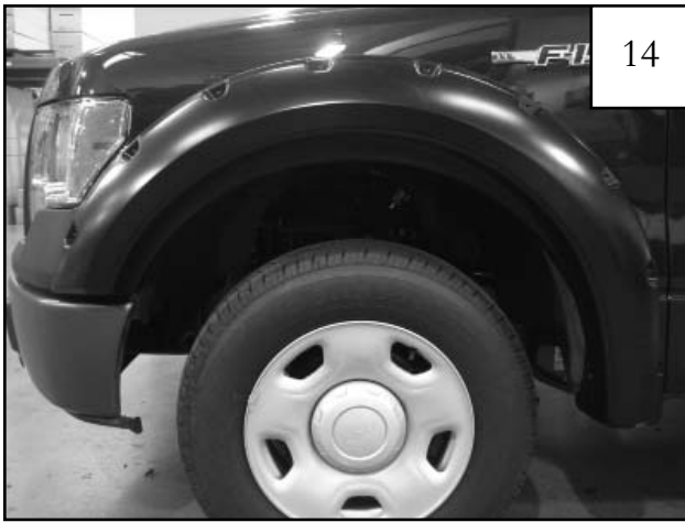
Completed front flare installation.
