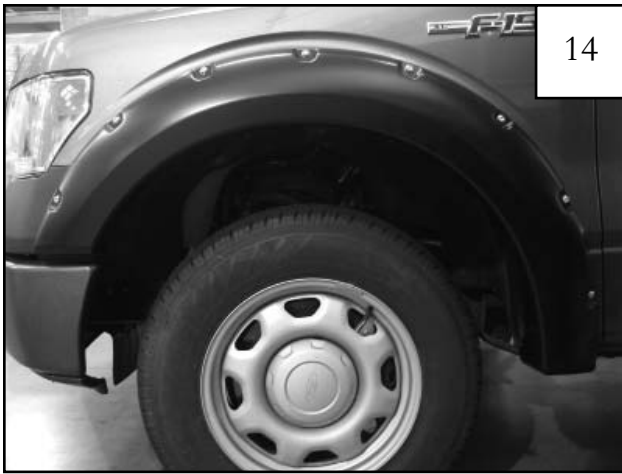
Completed front flare installation.
