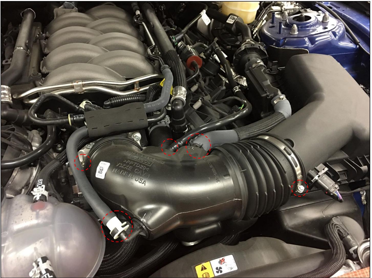
Figure 8 – Intake Air Tube Removal
