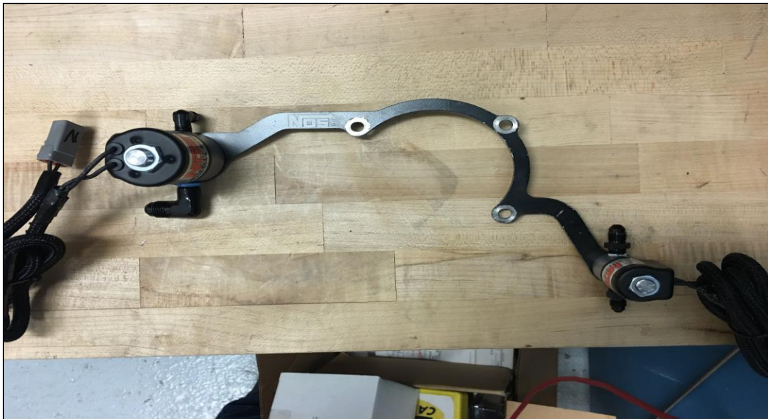
Figure 6 – Solenoid Bracket Assembly
