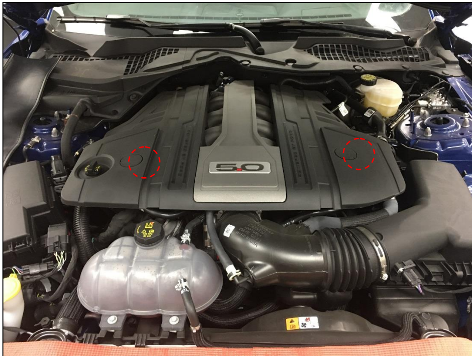
Figure 7 – Engine Cover Removal
