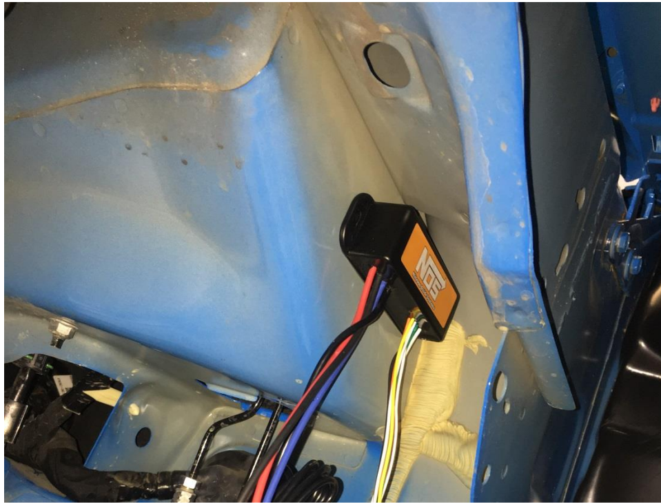
Figure 16 – Mini 2-Stage Mounting Location
