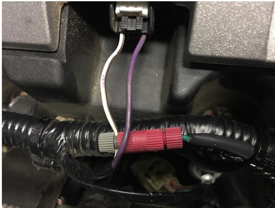
Figure 18 – Tach Signal Wire Connection
