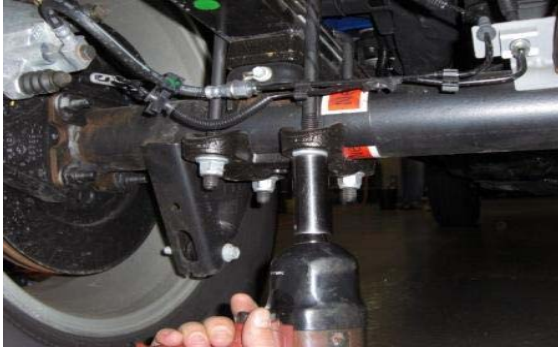
5. Loosen and remove factory u-bolt hardware.
