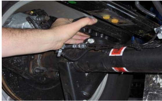
7. 4WD: Lower axle enough to remove factory block.
