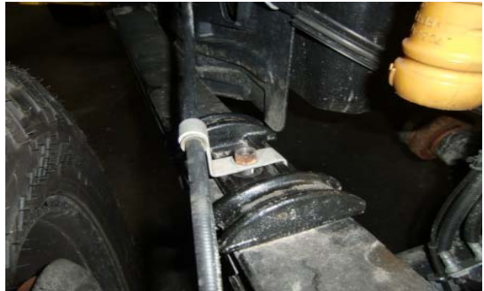
9. Remove e-brake bracket from upper u-bolt plate.
