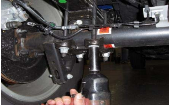
5. Loosen and remove factory u-bolt hardware.
