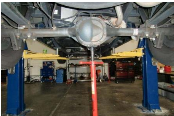
1. Raise vehicle at frame and support axle with jack.
