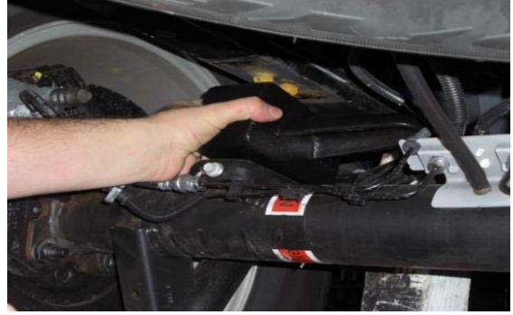
8. Install lift block if you don't have an Add-a-Leaf.
