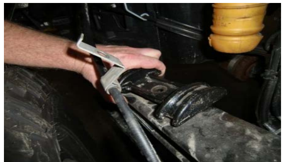
11. Remove upper u-bolt mounting plate and overload spring.
