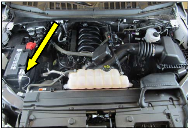
1. Disconnect the negative battery terminal.
