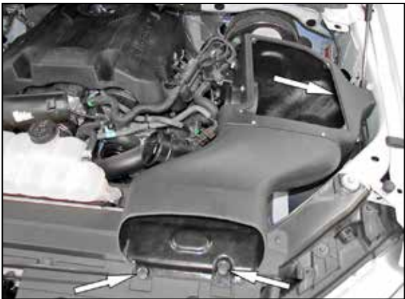
9. Install the AIRAID® air filter assembly into the vehicle and secure it to the inner fender and core support with the hardware and retaining clips provided.
