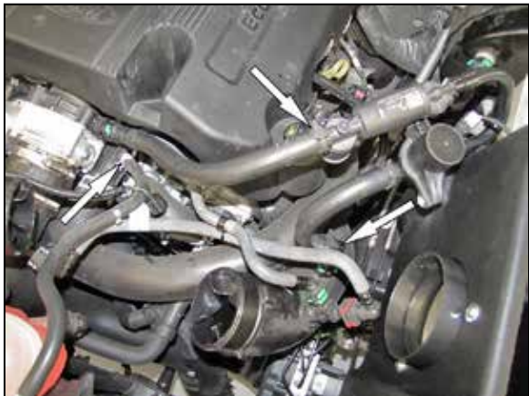
15. Install the modified crank hoses onto the solenoid valves and turbo intake tubes.
