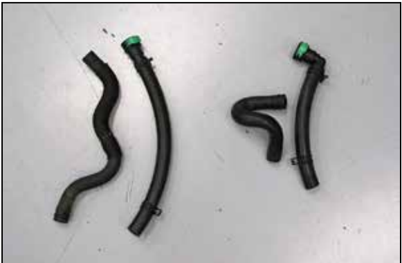
14. Remove the fittings from the factory crank case vent hoses in step #10 and install them into the 8” and 12-1/2” long hoses as shown.
