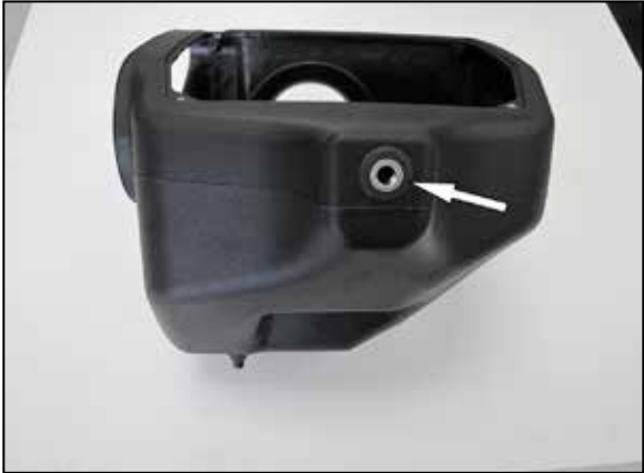
7. Install the provided grommet and support into the AIRAID® air filter housing as shown.
