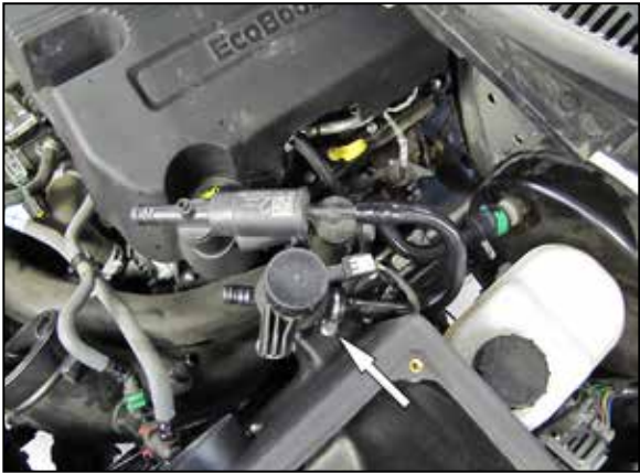
10. Remove the two crank case vent hoses from the solenoid valves and turbo inlet tubes and set aside. Using the provided clamp and hardware, secure the solenoid pack to the AIRAID® air filter housing. Rotate the brake booster hose where it attaches to the solenoid pack so the it lines up with the brake booster and does not cause a bind.
