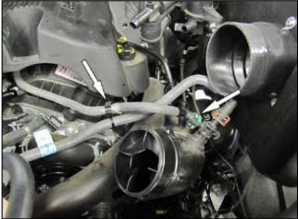
12. Route the line in front of the red EVAP line and reconnect to the fitting. Resecure the line retaining clip.
