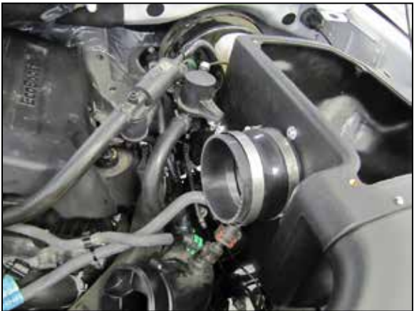
16. Install the coupler hose onto the filter adapter and secure with the provided hose clamp.
