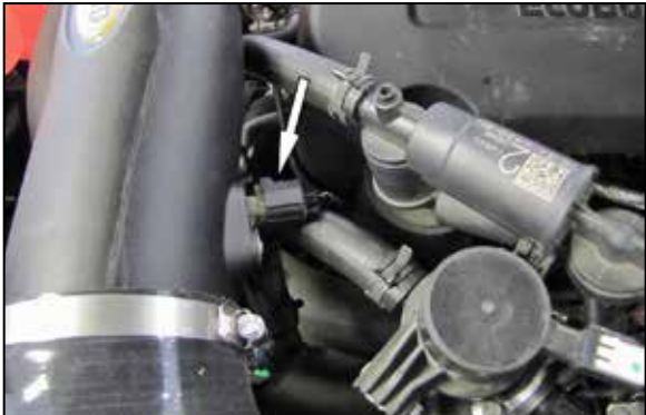
22. Using the provided extension harness, reconnect the inlet air temperature sensor.
