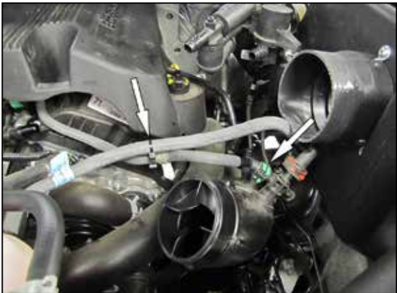
11. Disconnect the green EVAP connector and unhook the line from the retaining clip.
