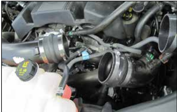
17. Install the two remaining coupler hoses onto the turbo inlet tubes and secure with the provided hose clamps.
