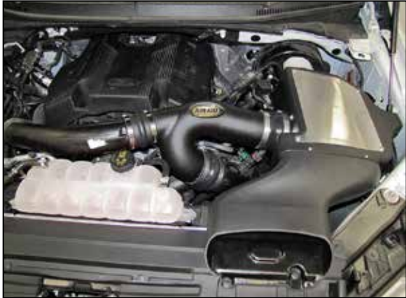
26. Double check your work! Make sure there is no foreign material in the intake path. Make sure all clamps, hoses, bolts, and screws are tight. Double check the hood clearance! Reconnect the negative battery cable!
