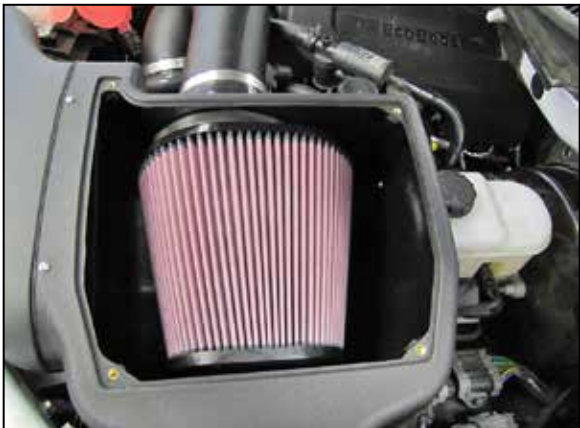
23. Install the AIRAID® air filter onto the adapter and secure with the provided hose clamp.
