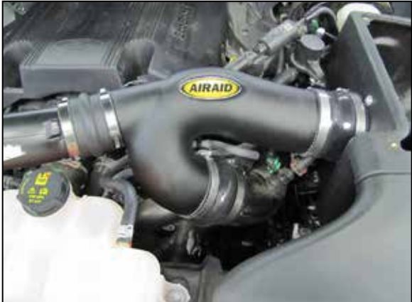
21. Install the intake tube into the turbo hose couplers and the coupler at the filter adapter. Adjust the tube for best fit and secure with the provided hose clamps.
