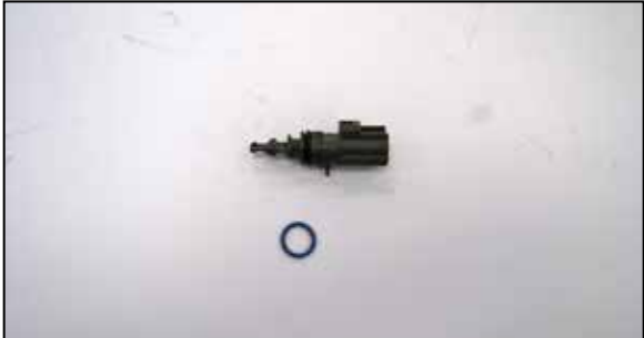
18. Remove the inlet air temperature sensor from the factory air filter housing and then remove the factory O-ring. Install the provided O-ring onto the inlet air temperature sensor.
