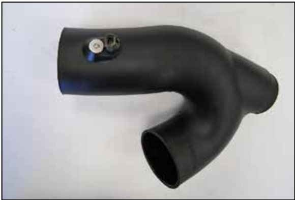
19. Install the inlet air temperature sensor into the AIRAID® intake tube and then secure with the provided hardware.
