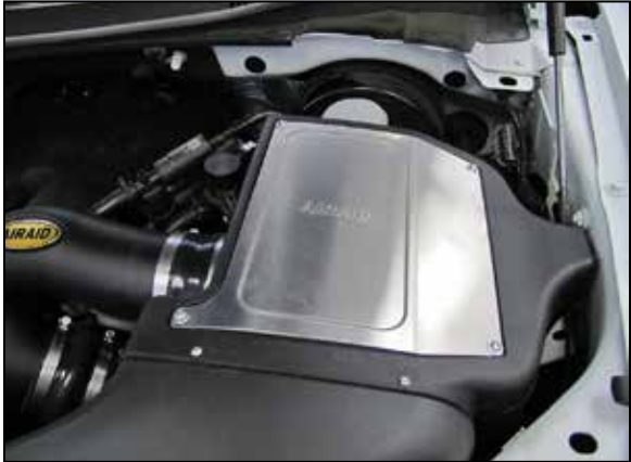
25. Install the air filter housing lid and secure with the provided hardware.
