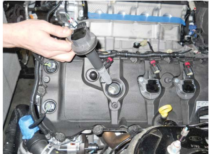
14. Using a 14 mm spark plug socket and a 6" extension, remove all eight (8) spark plugs.
