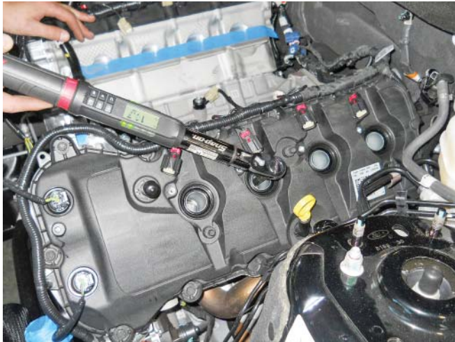
16. Install the spark plugs and torque to 14 Nm.
