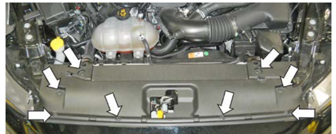
8. Release the eight (8) pushpin retainers by pulling the center pin and remove the radiator trim cover.
