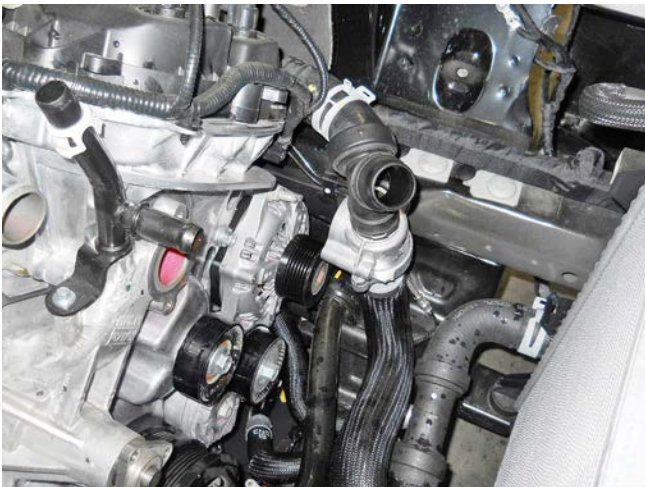
61. Remove the thermostat housing assembly and set it aside.
