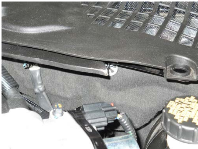
Exposed point on modified K-brace, shown installed
