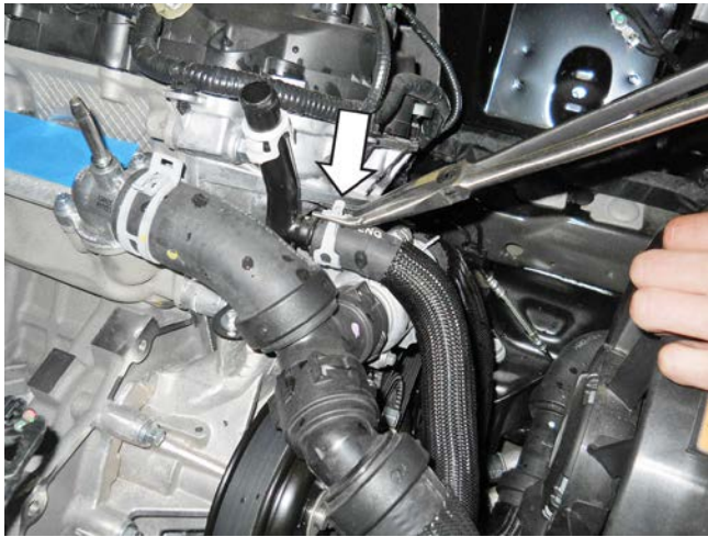
Degas hose from bottom of bottle
