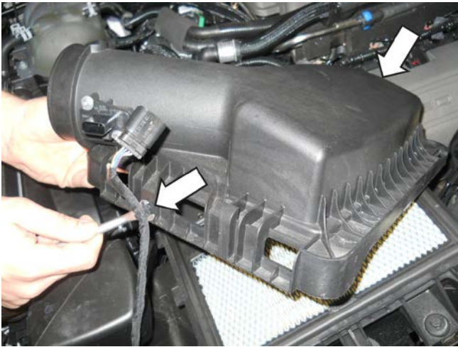
28. Remove the filter from the airbox. Remove the mounting bolt at the side of the airbox (10 mm socket). Pull up and remove the lower airbox from the vehicle.
