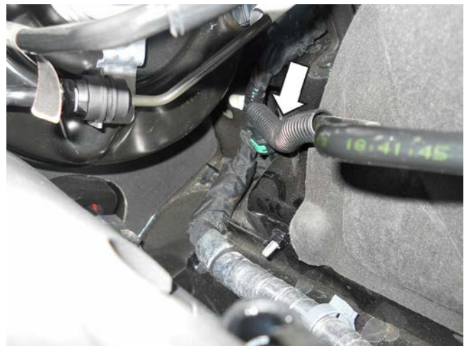
Disconnect green quick connect fitting
