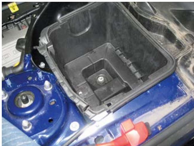
7. Remove the battery tray by first removing the three (3) 8 mm head bolts.
