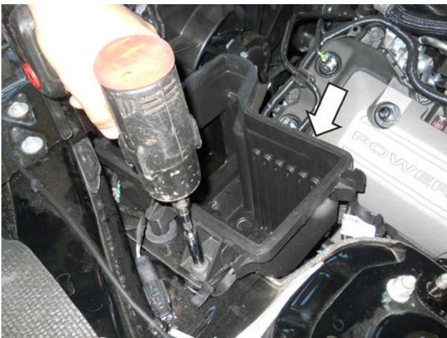
28. Remove the filter from the airbox. Remove the mounting bolt at the side of the airbox (10 mm socket). Pull up and remove the lower airbox from the vehicle.
