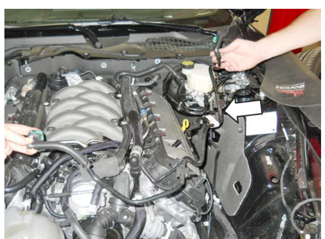
Disconnect green quick connect fitting
