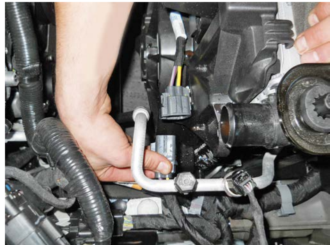
Fan shroud electrical connector
