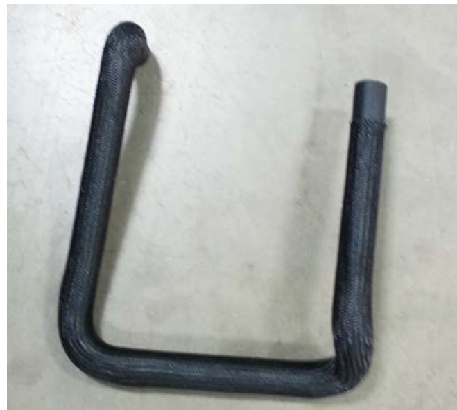
Intercooler pump outlet hose (1315-6K236)
