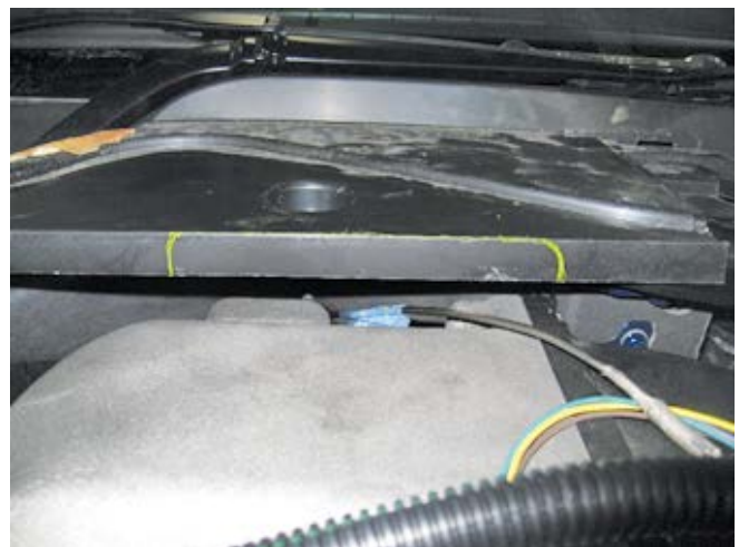
Exposed point on modified K-brace, shown installed
