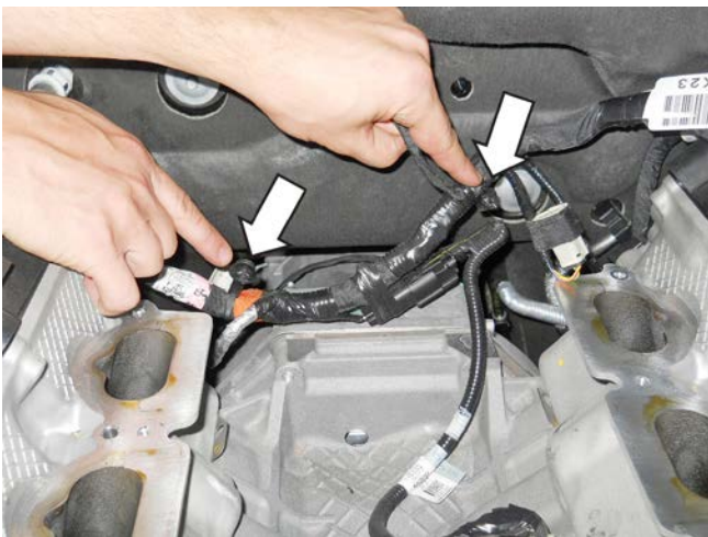
Pin retainers on harness
