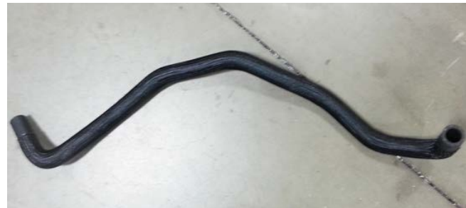
Intercooler pump inlet hose (1315-8D029)
