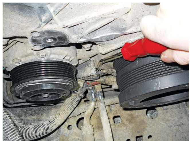
7. Remove the bolt. The line and wiring harness will need to be fastened to the tensioner bracket in a later step.
