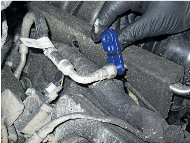
14. Disconnect the brake booster vacuum hose from the intake manifold. This port is located directly behind the throttle body.
