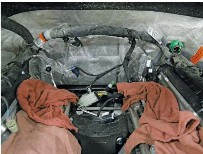
27. Clean the intake mounting surfaces and apply tape over the open intake ports to prevent engine contamination.
