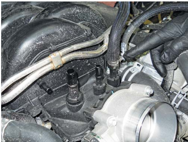
15. Disconnect the brake booster vacuum line from above brake master cylinder (only for 4x4).
