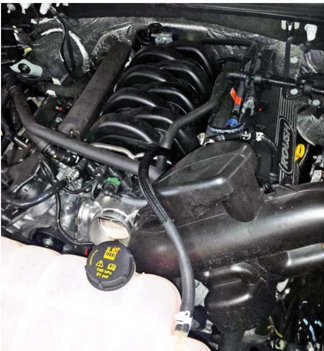
9. Remove the two (2) push clips retaining the dirty air inlet duct to the grill closeout.
