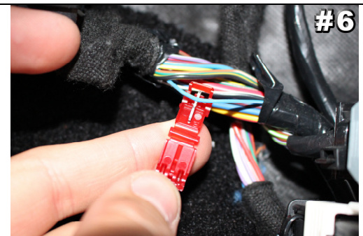
#6 Slide Gray w/ Purple Tracer wire into place and close wire tap firmly.
