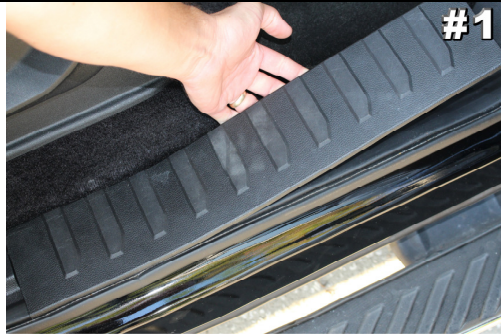
#1 Remove passenger side door sill plate carefully.
