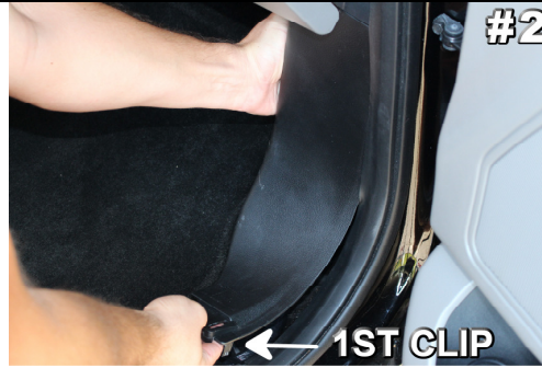
#2 Remove kick panel shown. First pull upward, then backward gently.
