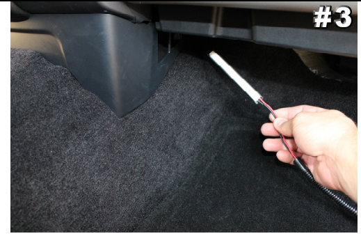
#3 Route driver side lamp behind center console toward driver side.
