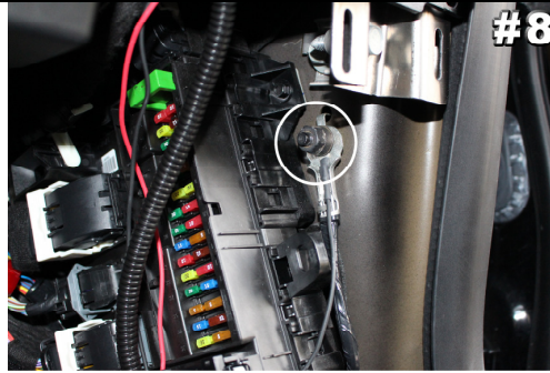
Attach black ground wire to the 13mm bolt circled above.
