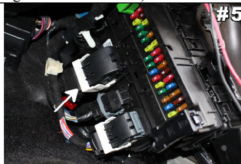
#5 Press release button/ tab while sliding bar to the side to unplug connector.
