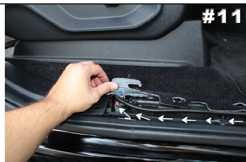
Route wiring along door sill and under carpet (wiring comes out under seat)
