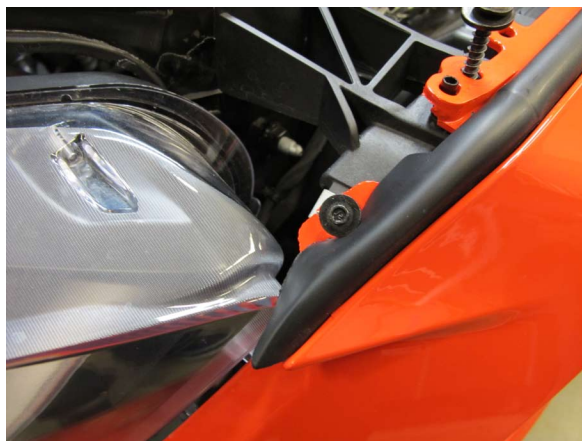
Fig. 1-c: Remove 5.5mm-Headed Fastener
