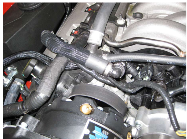
Fig. 4-c: Modified Passenger Side PCV Hose
