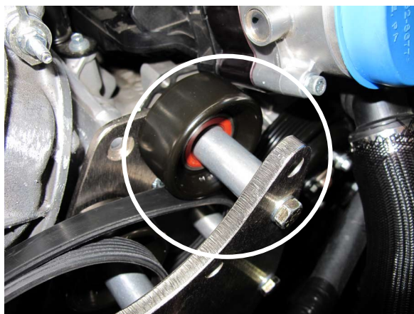
Fig. 3-m: Re-Install Upper Smooth Idler
