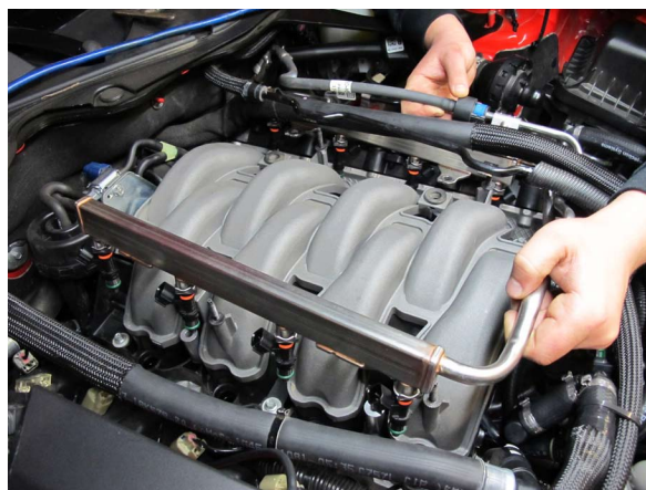
Fig. 6-c: Remove Fuel injector Rail Assembly
