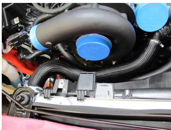
Fig. 7-c: Upper Radiator Hose (New Configuration)
