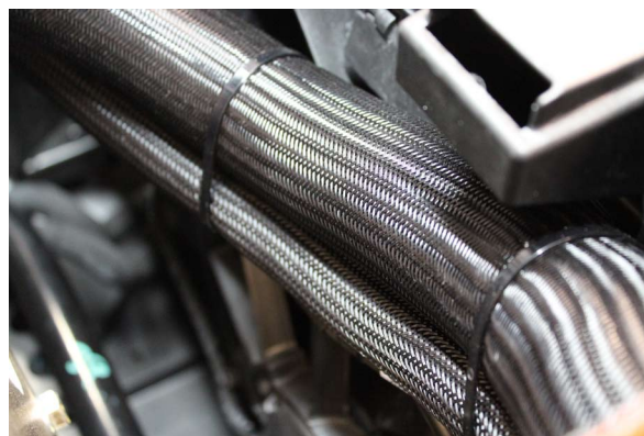
Fig. 7-o: 3/4" Coolant Hose Routing
