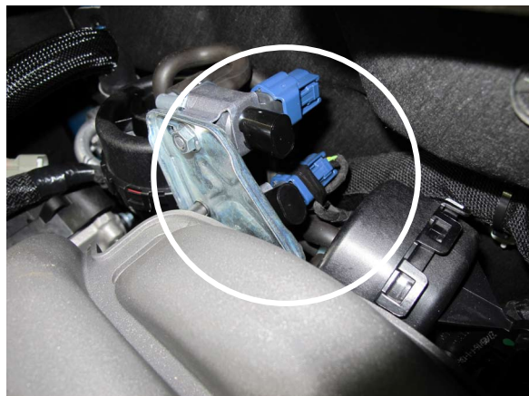
Fig. 8-p: Vented IMRC Solenoids
