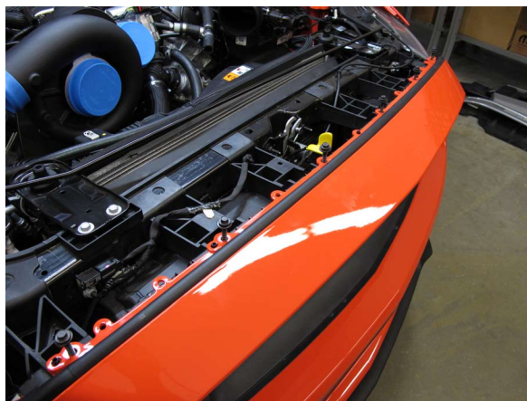
Fig. 1-b: Remove Bumper Cover Fasteners
