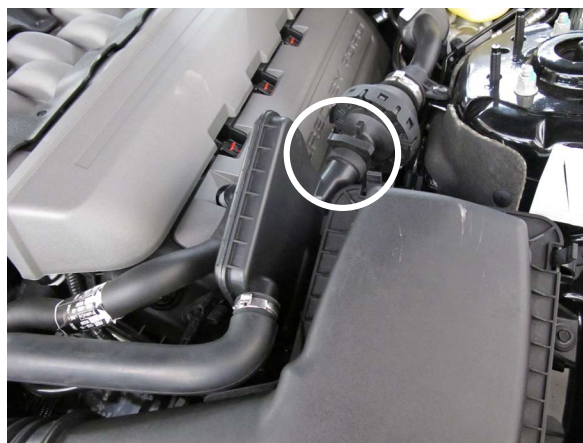
Fig. 1-n: Remove Interior Sound Tube
