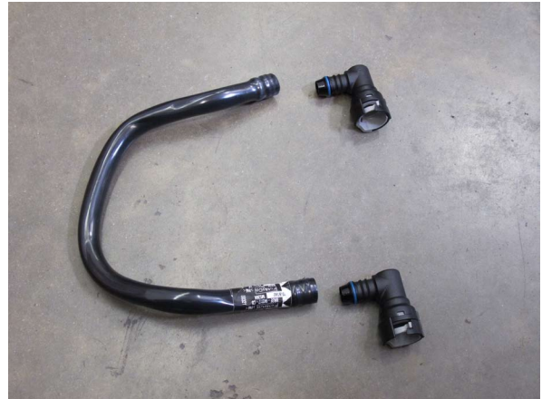
Fig. 4-a: OEM Passenger Side PCV Hose (Fittings Removed)
