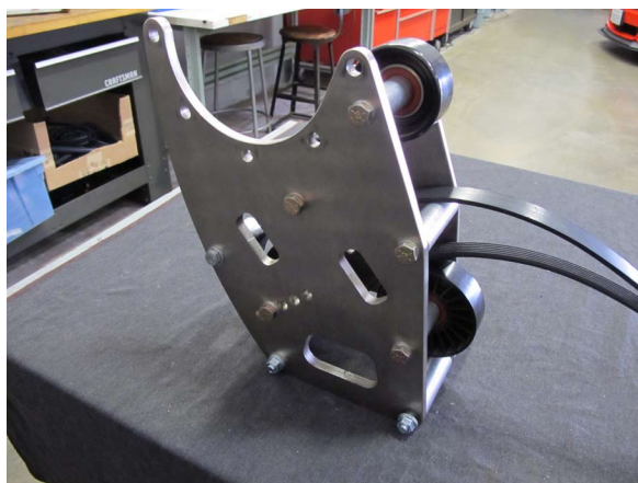
Fig. 3-c: Inspect Mounting Bracket Assembly
