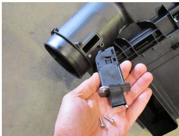
Fig. 1-s: MAF Insert (shown with OEM airbox removed)
