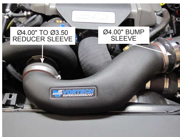
Fig. 8-b: Attach Air Inlet Duct To Air Box
