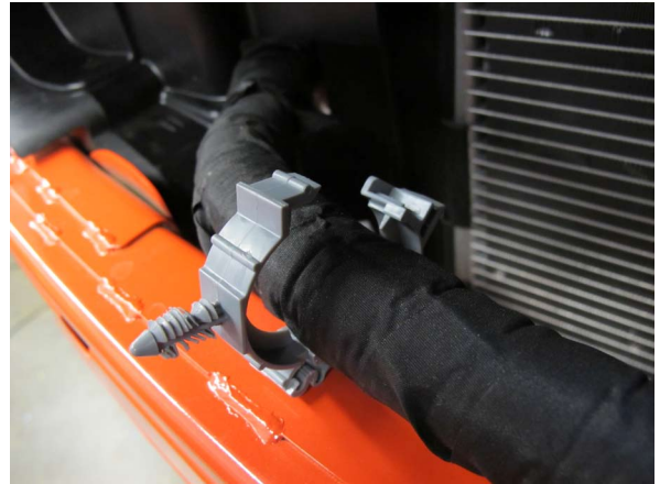
Fig. 1-j: Remove Gray Wire Harness Clips
