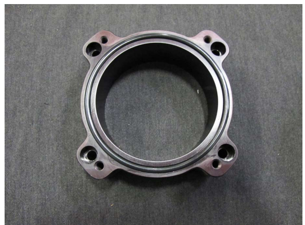
Fig. 3-u: Place O-Ring In Anodized Spacer
