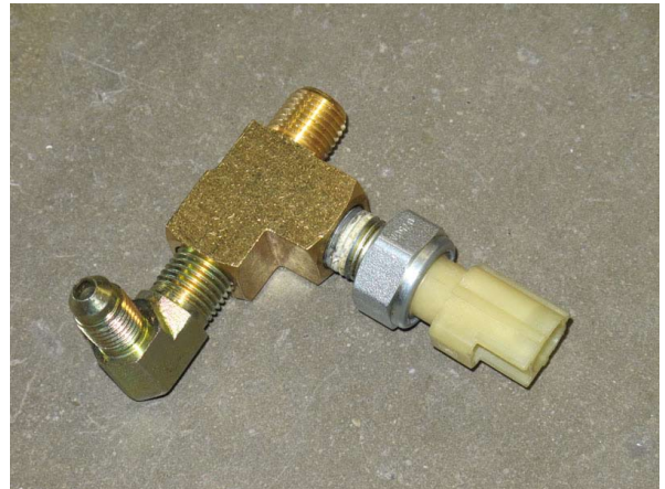
Fig. 11-e: Oil Feed Assembly (shown removed for clarity)
