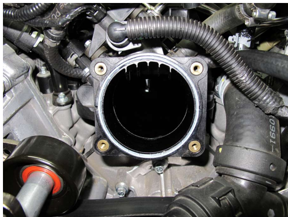
Fig. 3-v: Clean T-Body Flange & Verify O-Ring Placement
