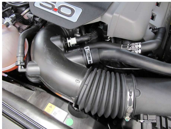
Fig. 1-m: Remove Intake Tube
