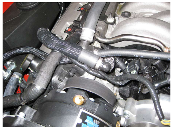
Fig. 4-c: Modified Passenger Side PCV Hose
