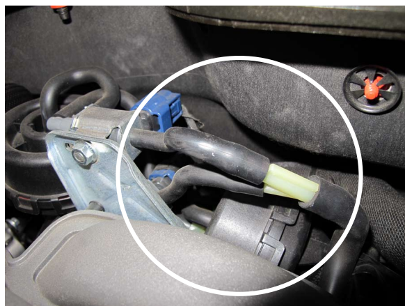
Fig. 8-d: Recirculating IMRC Solenoids
