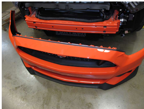
Fig. 1-h: Remove Front Bumper Cover
