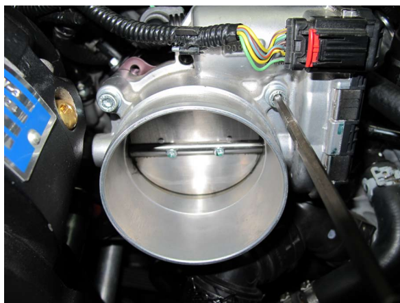
Fig. 3-w: Re-Install T-Body 180° From Original Orientation
