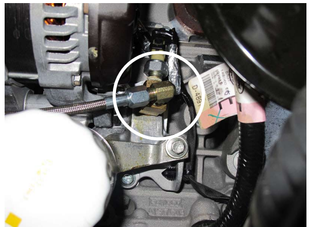
Fig. 11-f: Oil Feed Assembly Orientation
