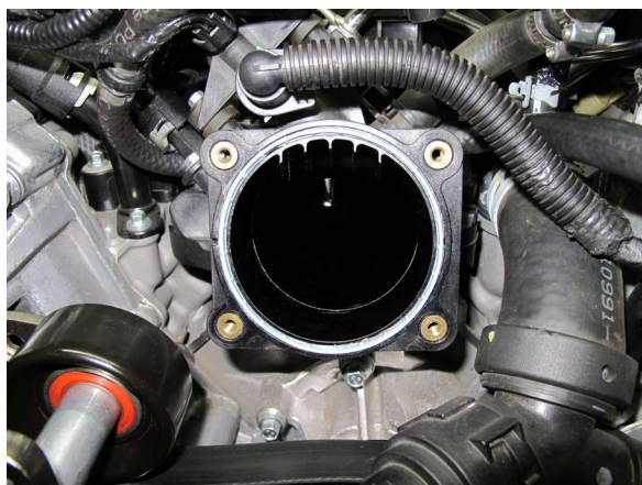
Fig. 3-v: Clean T-Body Flange & Verify O-Ring Placement
