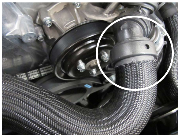
Fig. 7-b: Cut Plastic Hose Clamp
