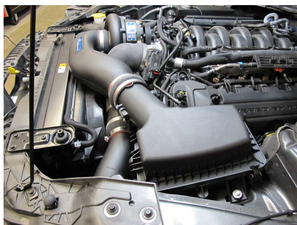
Fig. 8-c: Leave Air Inlet Assembly Loose At This Time
