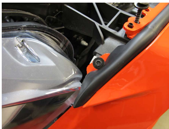
Fig. 1-c: Remove 5.5mm-Headed Fastener
