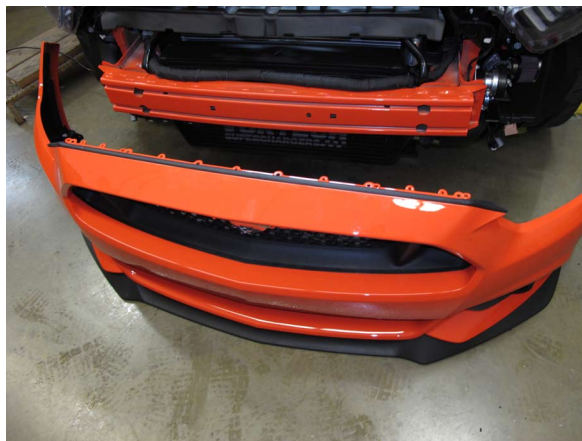
Fig. 1-h: Remove Front Bumper Cover
