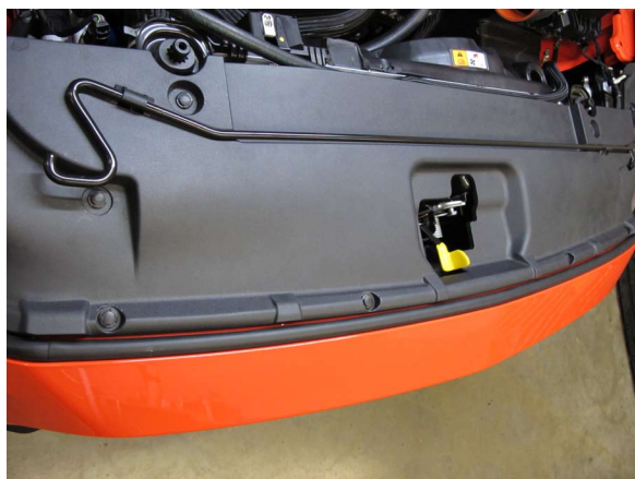
Fig. 1-a: Remove Plastic Cover
