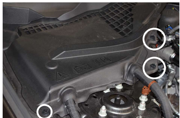
Fig. 2-c: Remove Battery Cover
