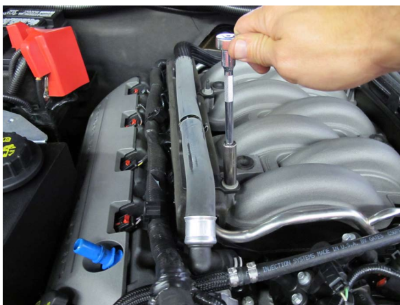
Fig. 6-b: Hose Guide Removal
