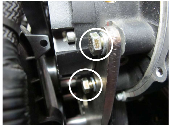
Fig. 3-q: Mount Supercharger To Bracket & Secure
