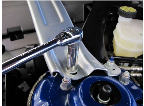
Fig. 2-d: Remove Strut Tower Brace
