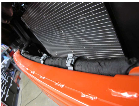
Fig. 1-i: Detach Wire Harness
