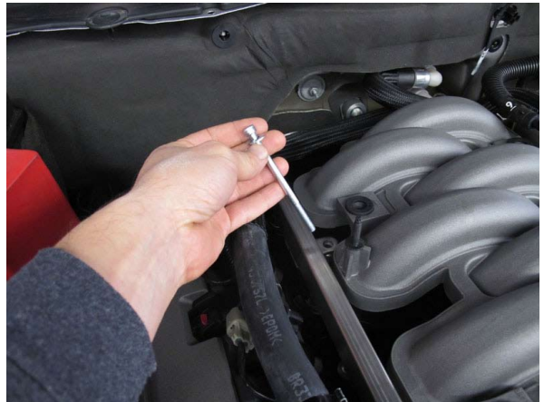
Fig. 6-e: Re-securing Fuel Rails
