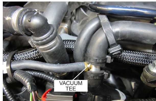
Fig. 9-b: Vacuum Tee Installation
