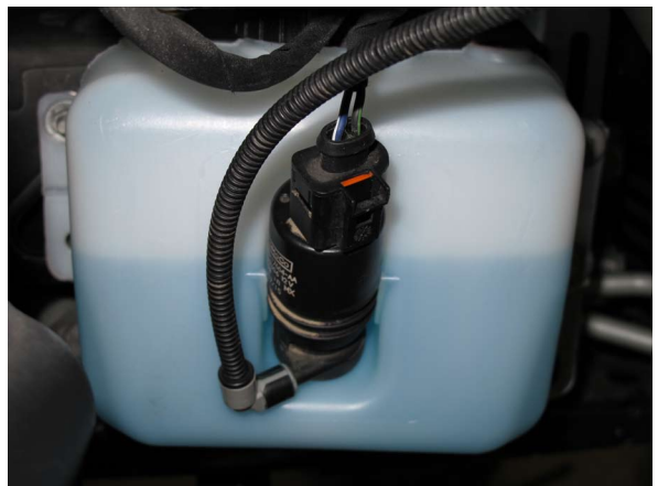
Fig. 10-l: Re-Install Windshield Washer Pump
