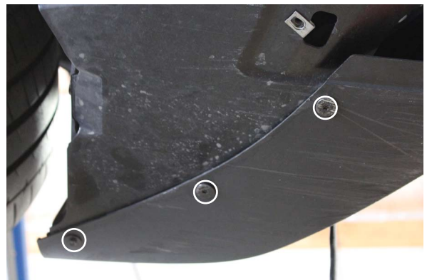
Fig. 1-f: Remove Screws Securing Front Bumper Corners
