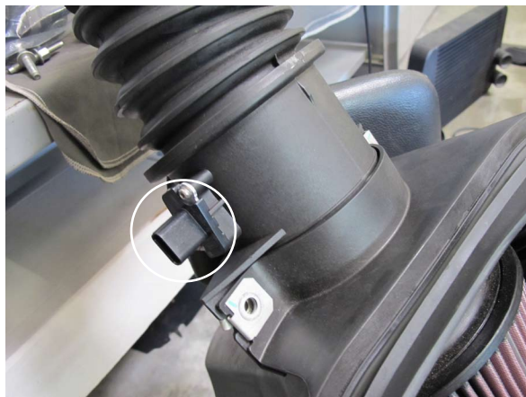
Fig. 1-s: MAF Insert (shown with OEM airbox removed)
