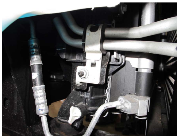
Fig. 10-b: Remove Transmission Cooler Lines From Mount
