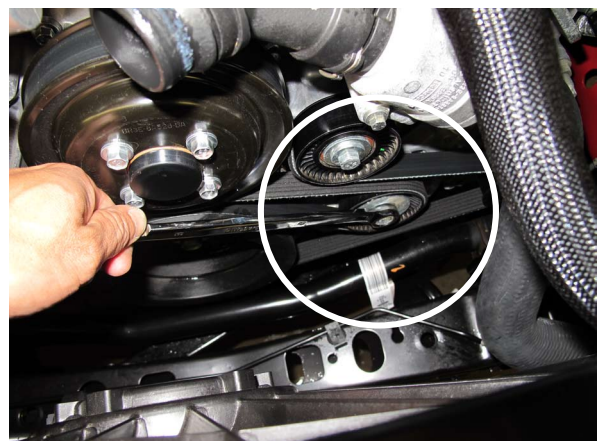
Fig. 1-r: Remove Accessory Drive Belt
