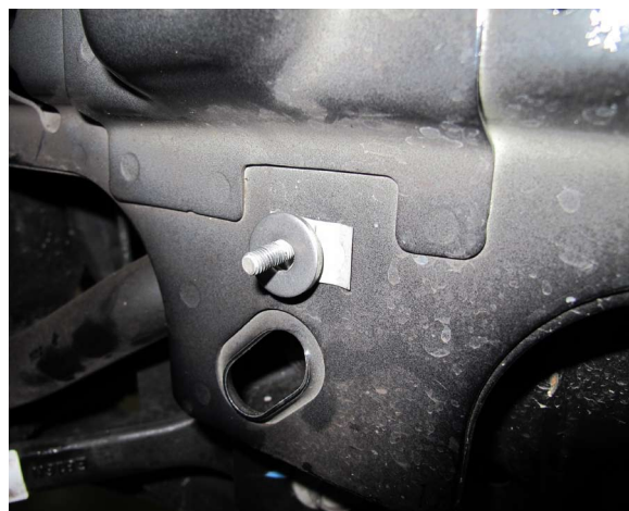
Fig. 10-i: Install 5/16 Washer To Mounting Stud
