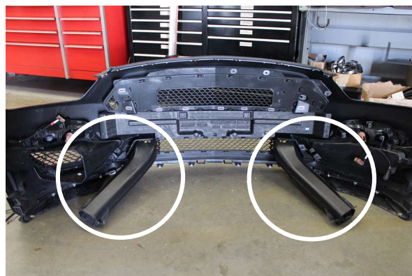
Fig. 5-n: Remove Brake Cooling Ducts
