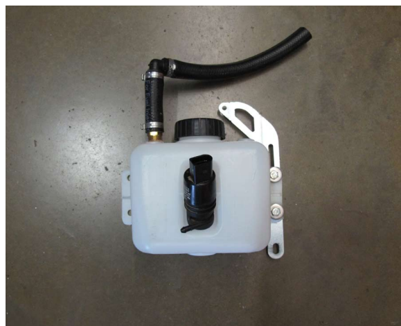
Fig. 10-h: Assemble Windshield Washer Reservoir As Shown
