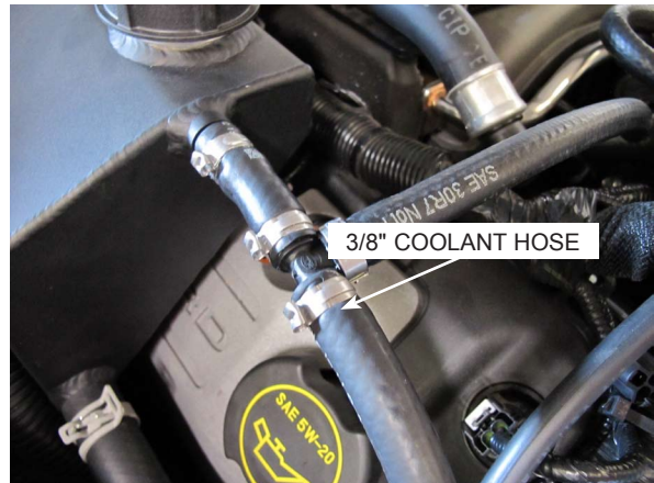
Fig. 7-m: Coolant Overflow Hose
