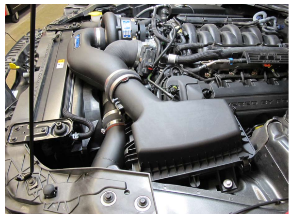
Fig. 8-f: Connect Inlet Duct To Air Box
