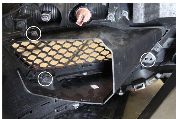
Fig. 5-o: Remove Oil Cooler Duct
