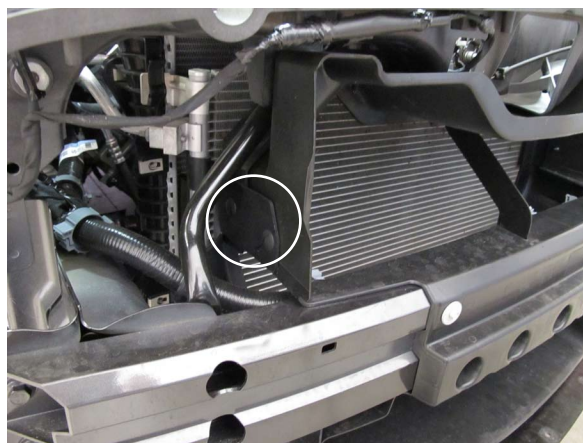
Fig. 1-i: Remove Plastic Fasteners
