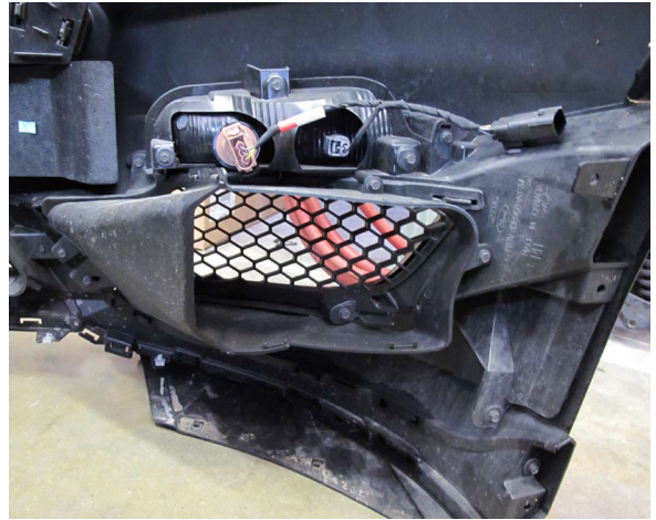
Fig. 10-m: Remove Transmission Cooler Duct
