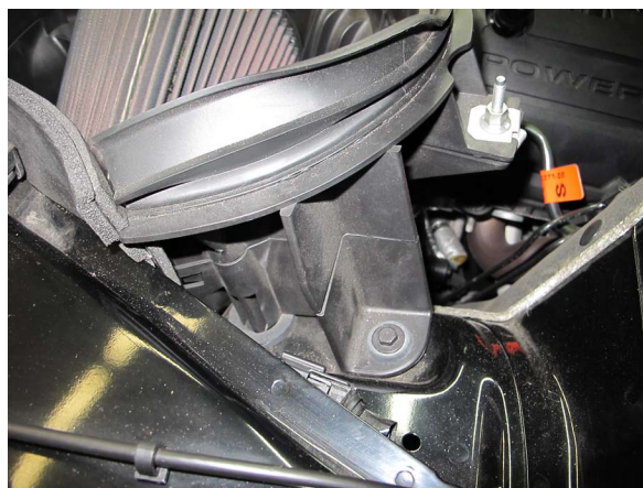
Fig. 1-n: Unplug MAF & Remove Air Inlet Assembly
