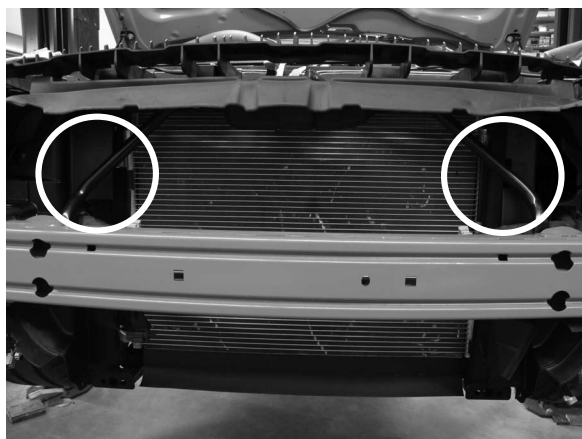
Fig. 5-a: Remove Front Braces
