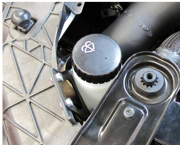
Fig. 10-g: Mount Remote Fill Bracket
