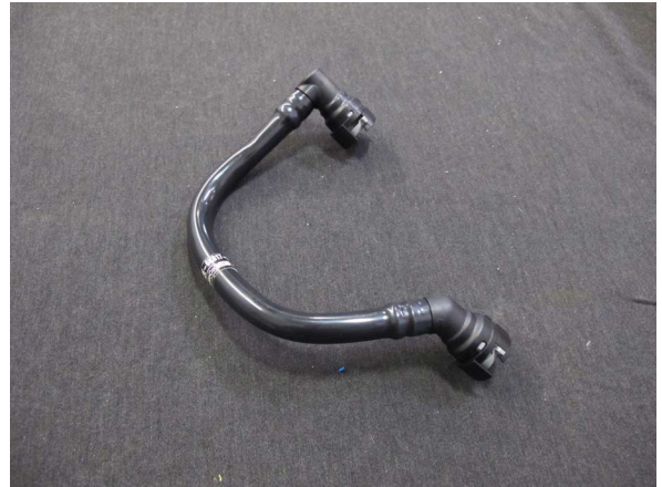
Fig. 4-a: OEM Passenger Side PCV Hose (Fittings Removed)
