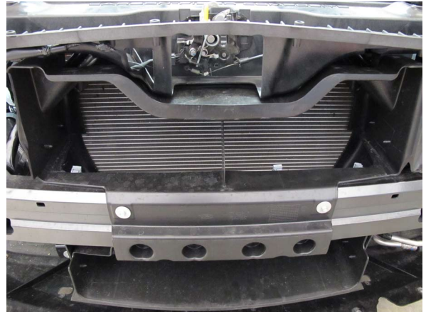
Fig. 1-j: Remove Radiator Shroud
