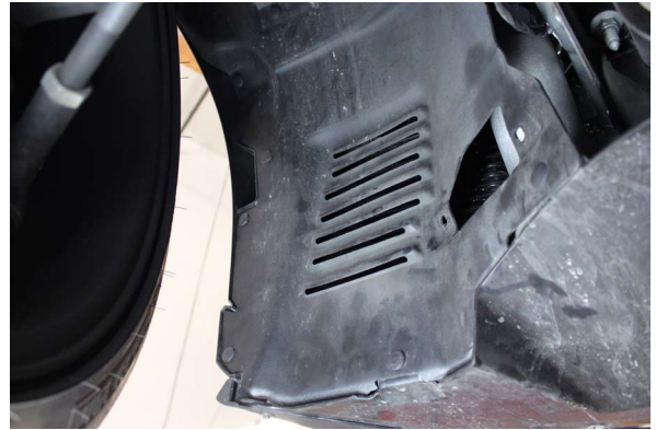
Fig. 1-d: Remove Fender Liner Fasteners
