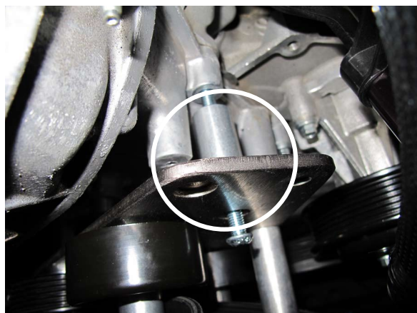
Fig. 3-j: Secure Top Of Rear Mounting Plate
