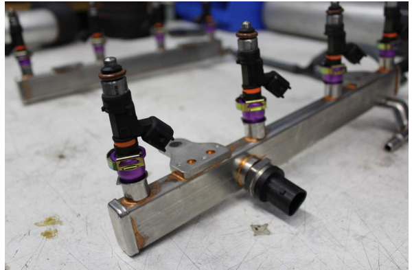
Fig. 6-d: Fuel Rail / Injector Assembly Detail
