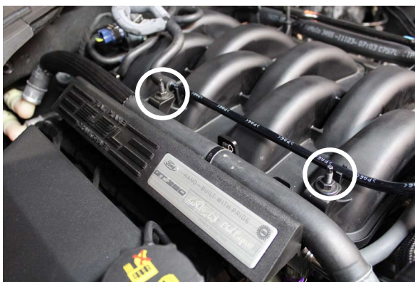
Fig. 6-b: Hose Guide Removal
