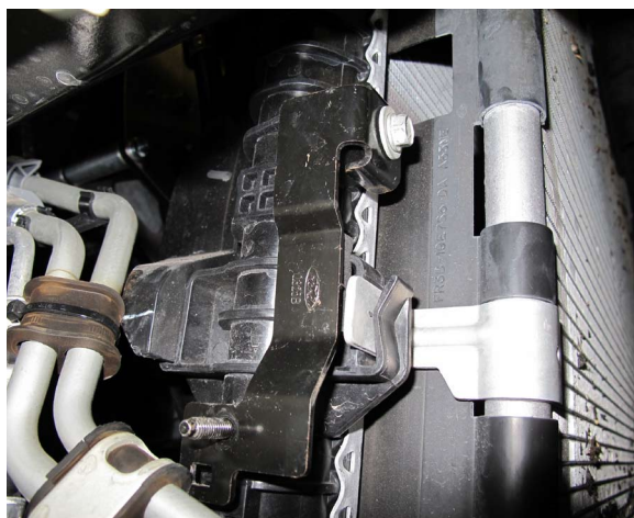
Fig. 10-c: Remove Transmission Cooler Lines Mount From Radiator
