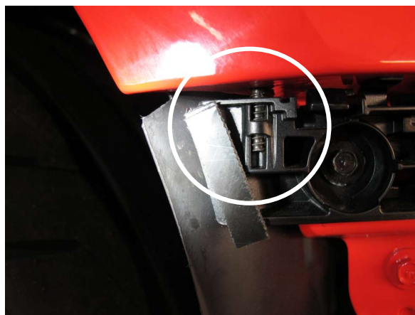
Fig. 1-h: Bumper Corner Fastener (Bumper Removed)
