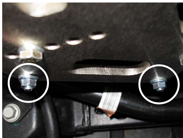
Fig. 3-l: Secure Lower Mounting Bracket Fasteners
