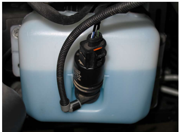
Fig. 10-l: Re-Install Windshield Washer Pump
