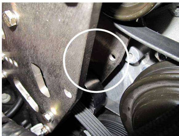
Fig. 3-n: Temporarily Remove Spacer (Circled)
