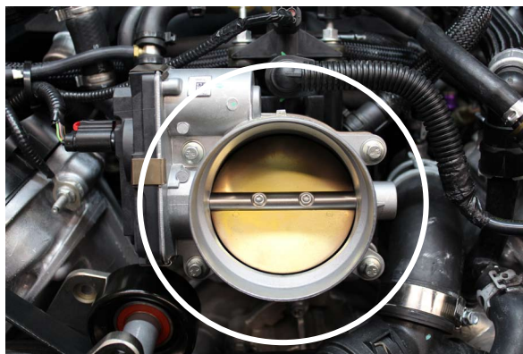
Fig. 1-t: Remove Throttle Body
