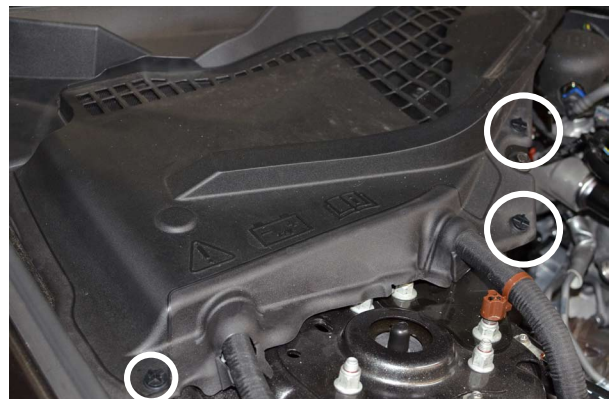
Fig. 2-c: Remove Battery Cover
