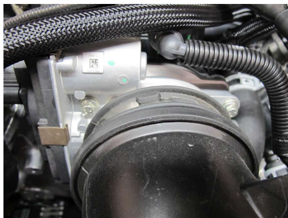
Fig. 1-m: Loosen Hose Clamp & Detach Breather Hoses
