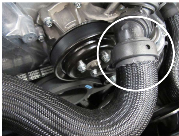
Fig. 7-b: Cut Plastic Hose Clamp
