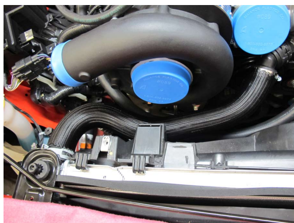
Fig. 7-c: Upper Radiator Hose (New Configuration)
