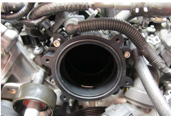
Fig. 3-u: Clean T-Body Flange & Verify O-Ring Placement
