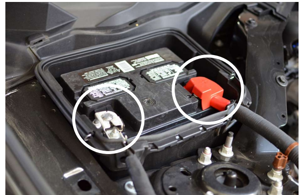
Fig. 2-e: Unplug Battery Leads
