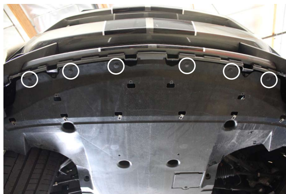
Fig. 1-g: Remove Front Belly Pan Screws
