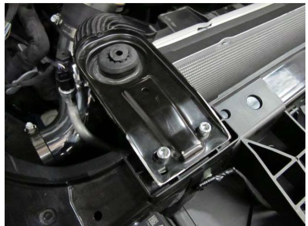
Fig. 4-av: Reinstall Modified Upper Radiator Brackets
