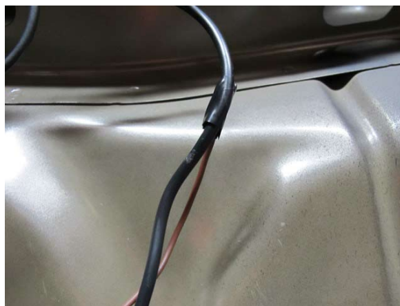
Fig. 6-n: Brown Wire (Unused)
