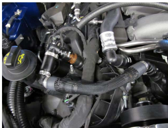
Fig. 7-e: Install PCV Assembly
