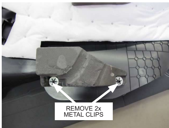
Fig. 6-i: Remove Foam Insulation Block
