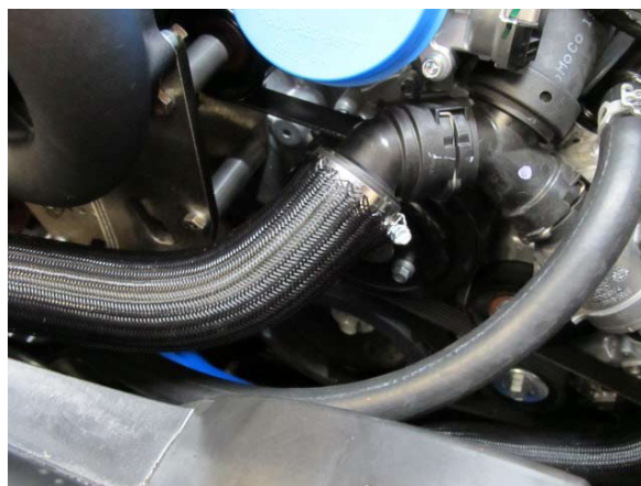
Fig. 3-l: Secure Quick-Release To Hose Using #24 Hose Clamp
