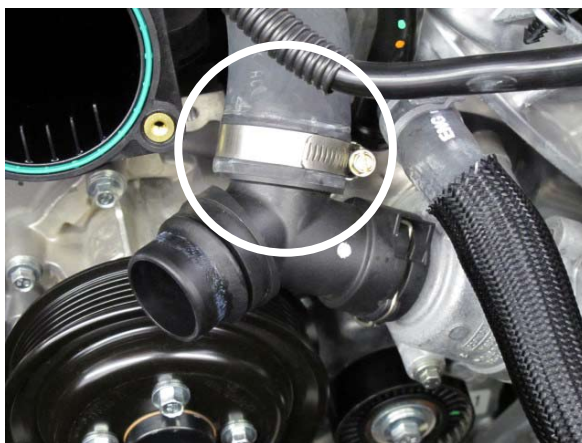
Fig. 3-h: Install #24 Hose Clamp
