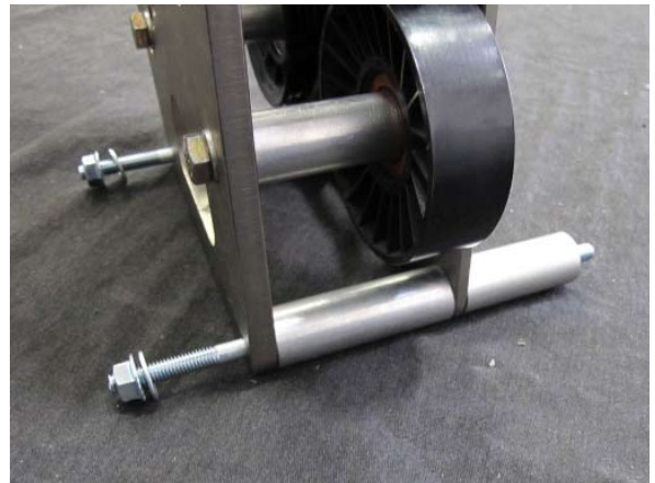
Fig. 2-h: Keep 2x 2.730" Spacers In Place
