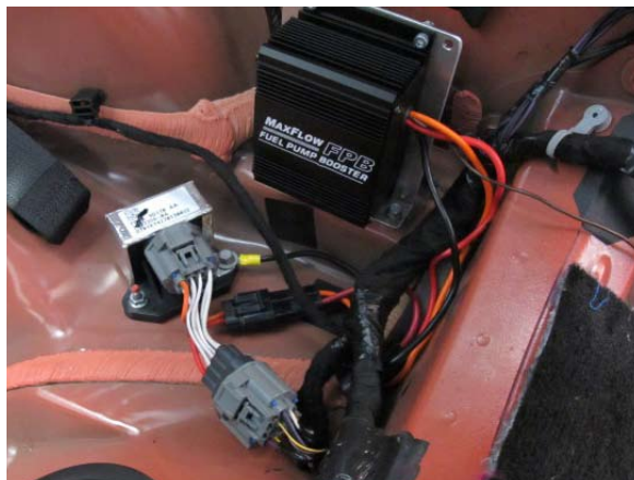
Fig. 6-m: Install Adapter Harness
