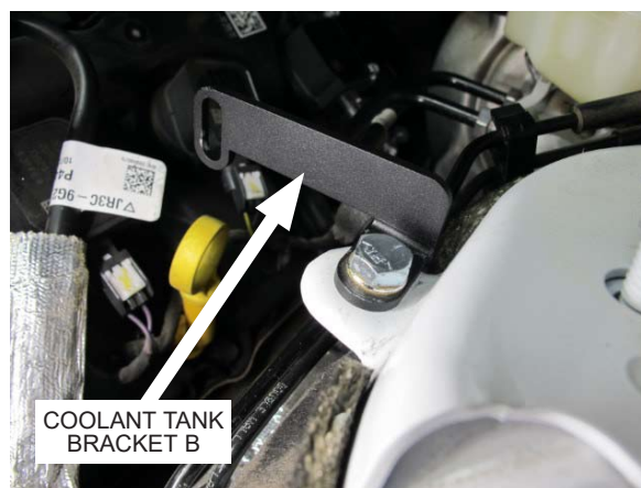
Fig. 3-q: Secure Coolant Tank Bracket B
