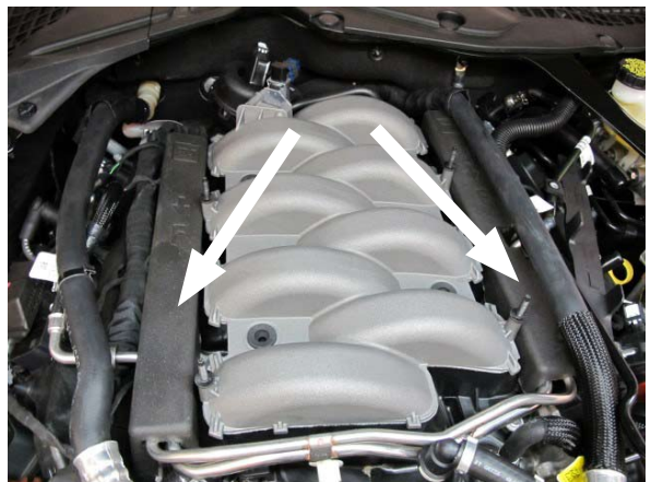
Fig. 5-c: Remove Fuel Injector Foam Insulation
