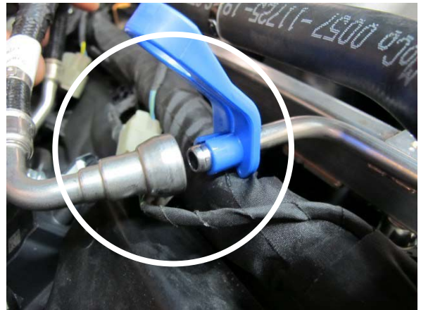
Fig. 5-g: Disconnect Direct Injection Fuel Line
