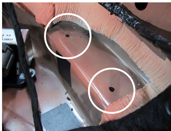
Fig. 6-k: Mark & Drill Mounting Holes
