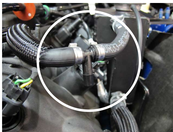
Fig. 3-x: Secure 3/8" Plastic Tee
