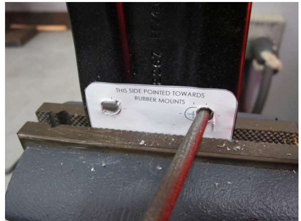
Fig. 3-d: Use Round File To Slot Hole
