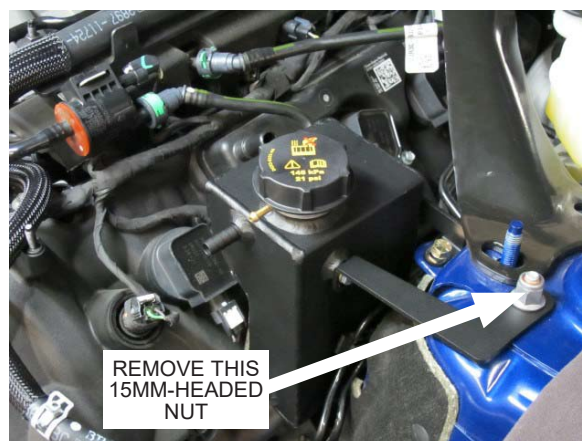
Fig. 3-r: Loosely Attach Coolant Tank
