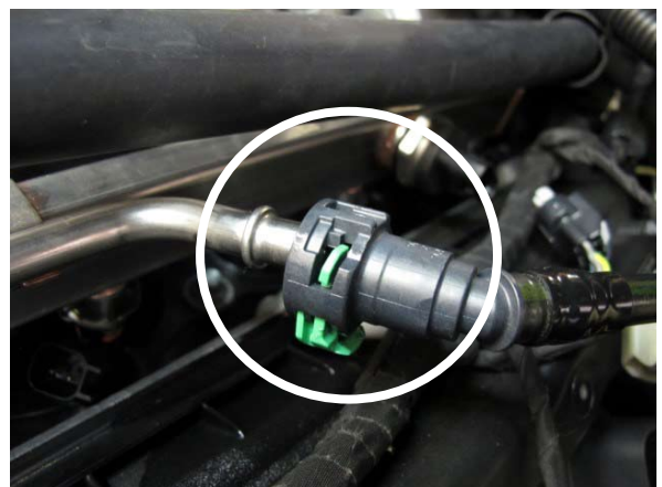
Fig. 5-f: Disconnect Low Pressure Fuel Feed Line
