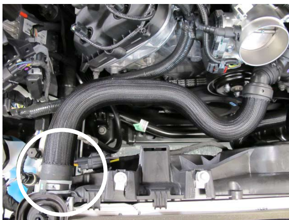
Fig. 3-i: Upper Radiator Hose (OEM Configuration)
