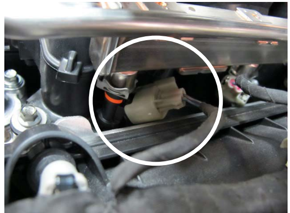
Fig. 5-d: Disconnect Fuel Injectors
