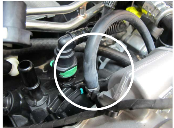
Fig. 4-ar: Attach Vacuum Hose To 1/4" Fitting
