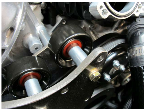
Fig. 2-m: Install Previously Removed Smooth Idler Pulley
