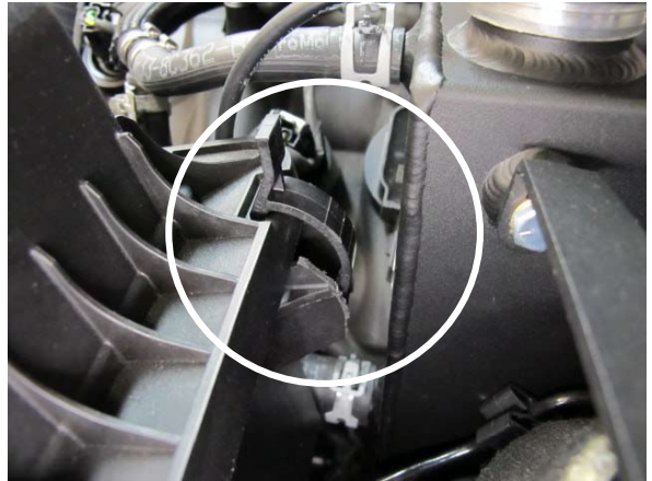
Fig. 7-g: Trim Air Box As Necessary
