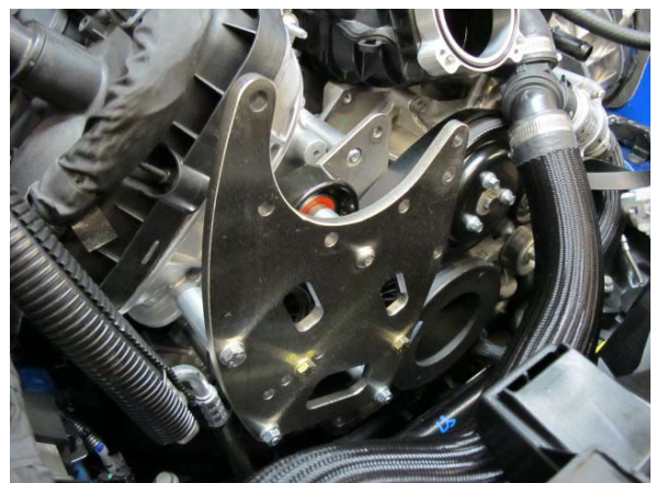
Fig. 2-i: Install Supercharger Mounting Bracket Assembly
