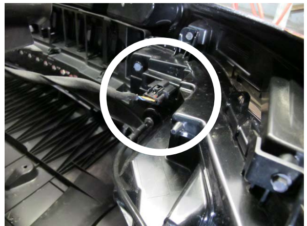
Fig. 1-l: Unplug Bumper Lights
