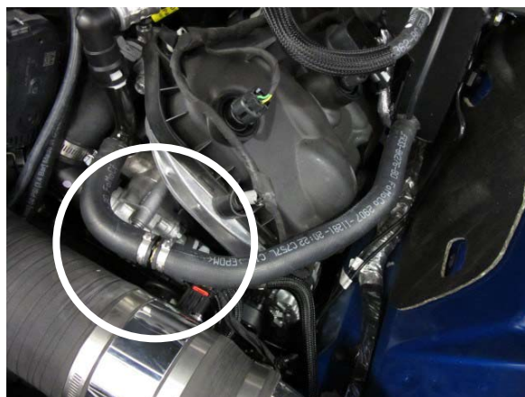
Fig. 3-v: OEM 3/4" Coolant Hose (Modified)
