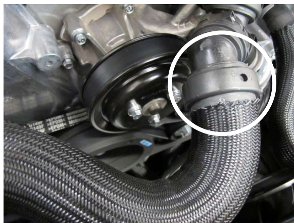
Fig. 3-j: Remove Plastic Hose Clamp
