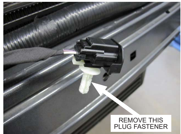
Fig. 4-z: Remove Plug Retainer
