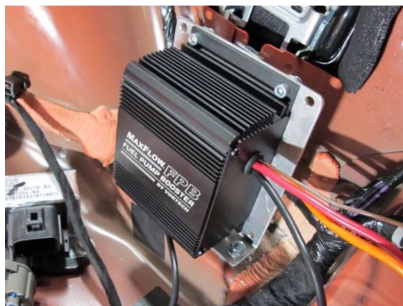
Fig. 6-l: Mount Fuel Pump Booster
