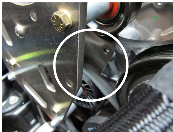
Fig. 2-n: Remove This 1x 2.730" Spacer & Set Aside
