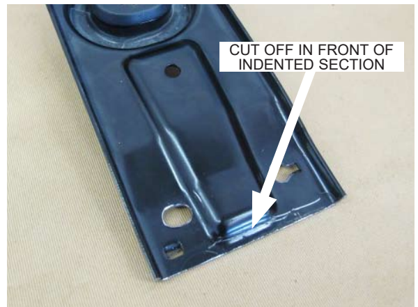
Fig. 3-e: Cut The Upper Radiator Bracket As Shown
