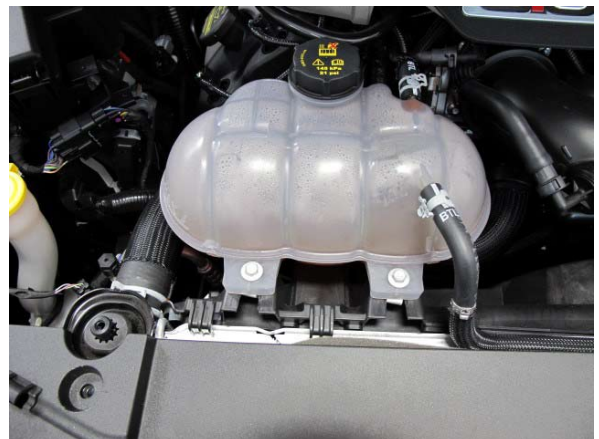
Fig. 1-x: Remove Coolant Reservoir
