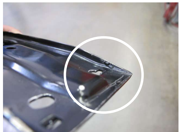
Fig. 3-f: Grind Down Raised Edges To A Taper
