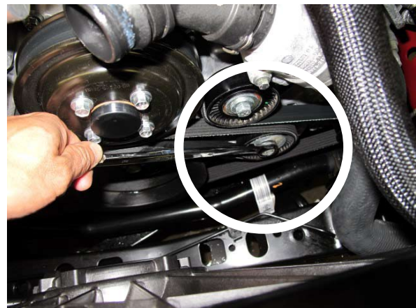
Fig. 1-z: Remove Accessory Drive Belt
