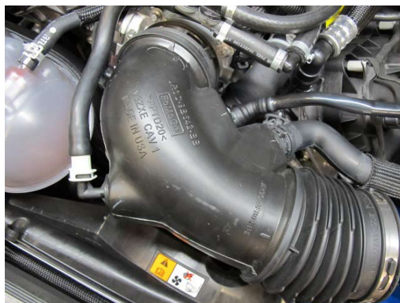
Fig. 1-u: Remove OEM Air Inlet
