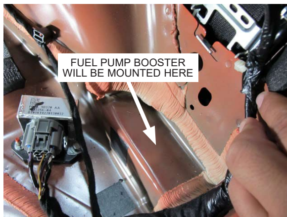
Fig. 6-j: Fuel Pump Booster Mounting Location
