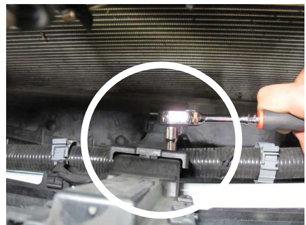
Fig. 1-r: Remove 2x 5.5mm-Headed Fasteners
