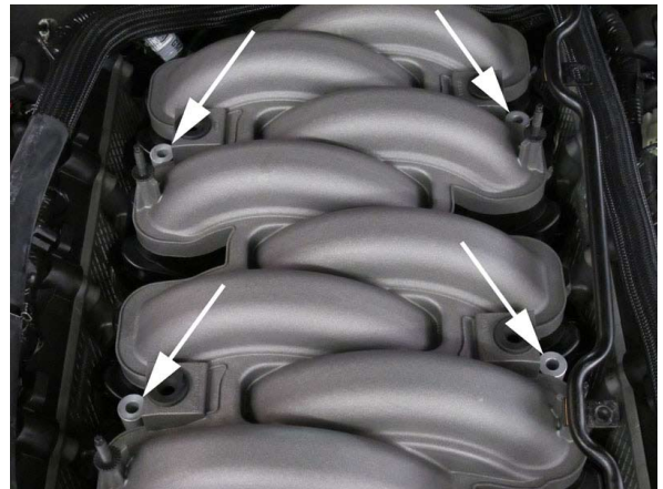
Fig. 5-n: Install Provided Fuel Rail Spacers
