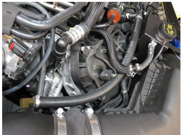
Fig. 7-i: Attach Breather Hose To Air Inlet
