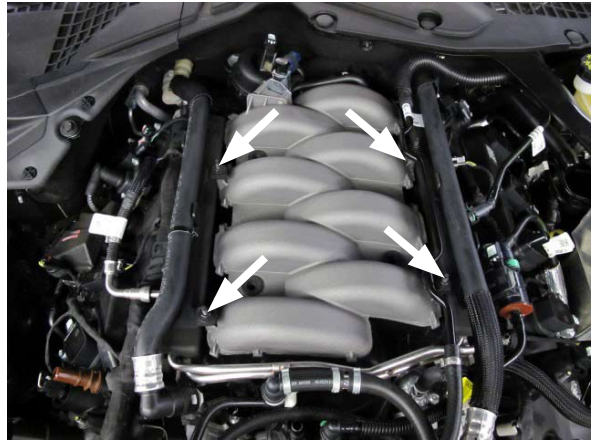
Fig. 5-a: Remove Fuel Injector Rail Fasteners
