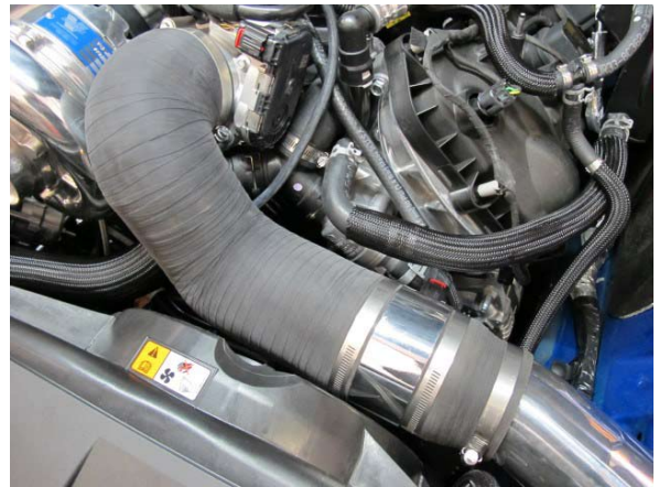
Fig. 4-aq: Secure All Hose Clamps
