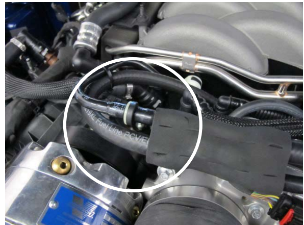
Fig. 7-k: Install 24" Length Of 3/8" Hose
