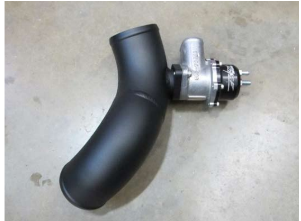
Fig. 4-ah: Install Bypass Valve (Automatic Transmission Vehicles)
