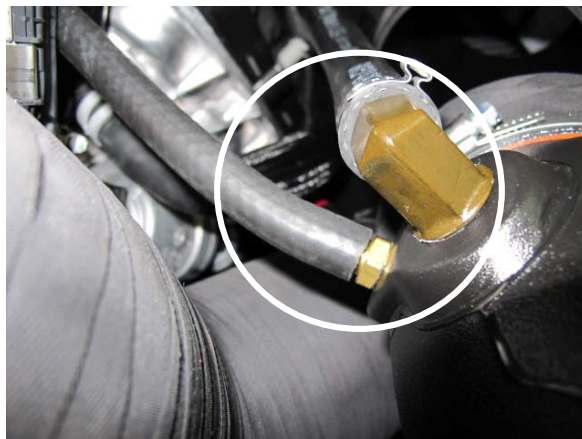
Fig. 7-m: Install 3/8" Hose, Then Secure Air Inlet Tube
