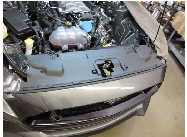
Fig. 1-d: Remove Radiator Support Cover
