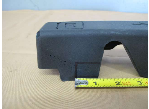
Fig. 5-m: Modify Passenger Side Fuel Rail Cover
