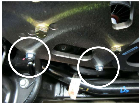
Fig. 2-l: Install 2x M8 Nuts & 2x 5/16" Washers
