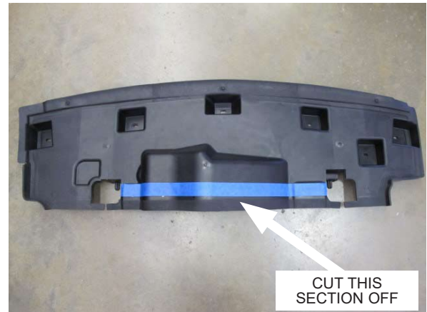
Fig. 4-ab: Modify Upper Radiator Shroud
