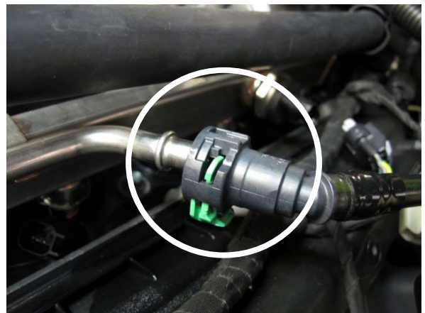
Fig. 5-f: Disconnect Low Pressure Fuel Feed Line
