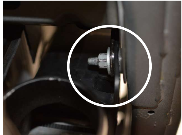
Fig. 4-y: Secure Charge Air Cooler
