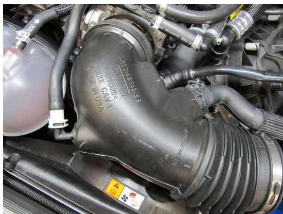
Fig. 1-u: Remove OEM Air Inlet
