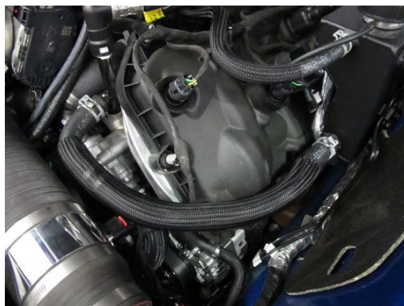
Fig. 3-w: Secure Modified OEM 3/4" Coolant Hose
