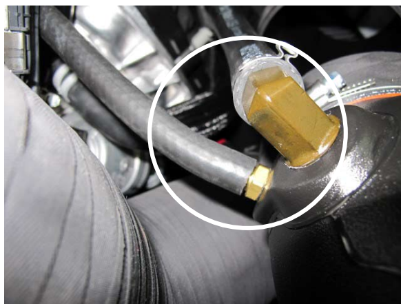
Fig. 7-m: Install 3/8" Hose, Then Secure Air Inlet Tube
