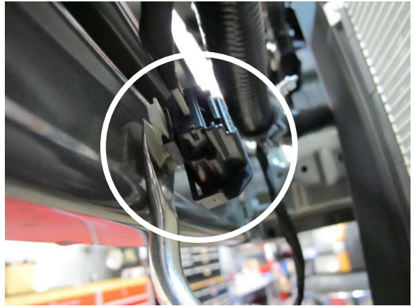
Fig. 4-n: Remove Unused Plug From Front Bumper Support
