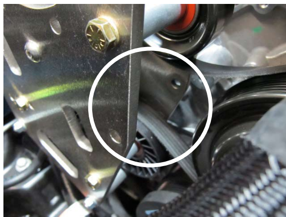
Fig. 2-n: Remove This 1x 2.730" Spacer & Set Aside
