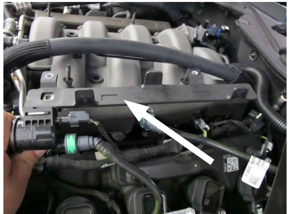
Fig. 5-b: Set Driver Side Heater Hose Guide Aside
