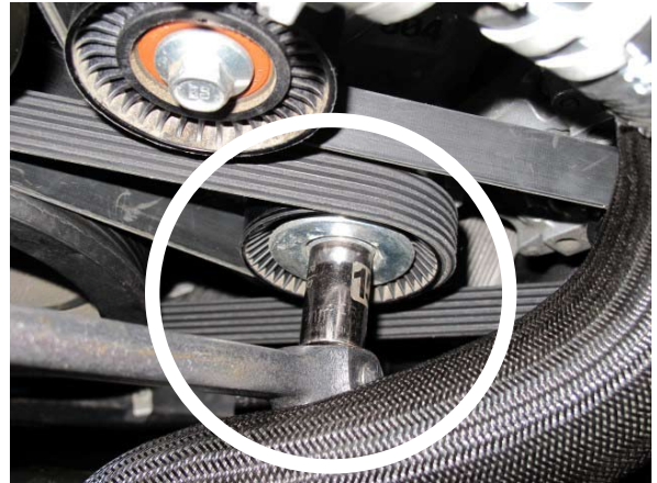
Fig. 2-s: Install Supercharger Drive Belt
