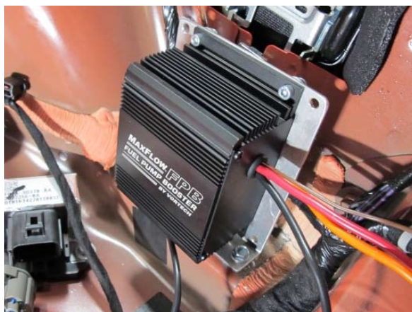
Fig. 6-l: Mount Fuel Pump Booster
