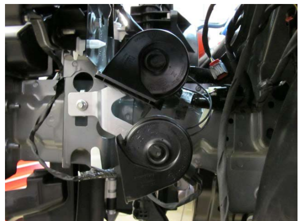
Fig. 4-ad: Remove Horn Assembly
