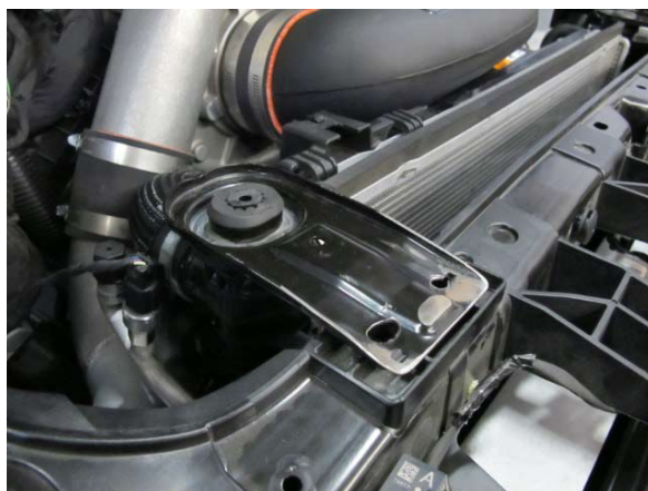
Fig. 3-g: Reinstall Modified Upper Radiator Brackets
