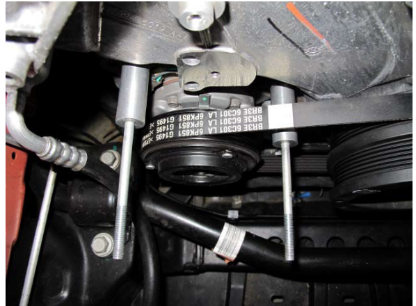
Fig. 2-g: Install 1x 2.058" & 1x 2.146" Spacers
