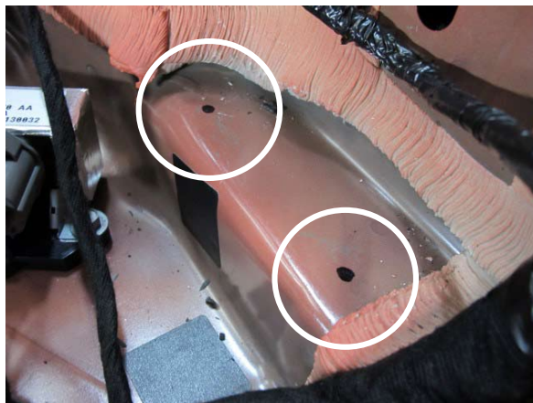
Fig. 6-k: Mark & Drill Mounting Holes
