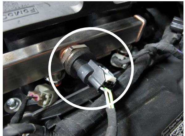
Fig. 5-e: Disconnect Fuel Rail Pressure Sensor
