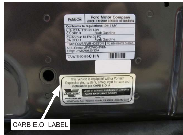
Fig. 8-b: Affix Emissions Label As Shown
