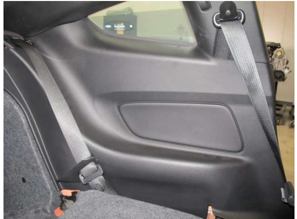
Fig. 6-p: Reinstall Driver Side Rear Interior Panel
