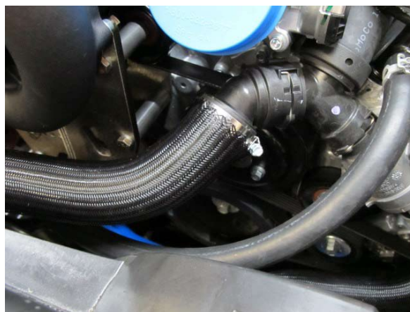
Fig. 3-l: Secure Quick-Release To Hose Using #24 Hose Clamp
