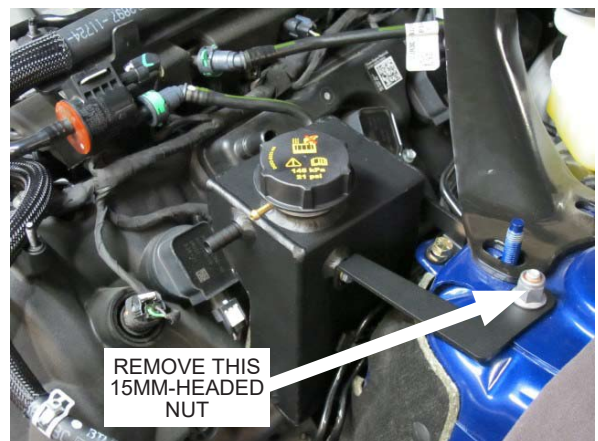
Fig. 3-r: Loosely Attach Coolant Tank
