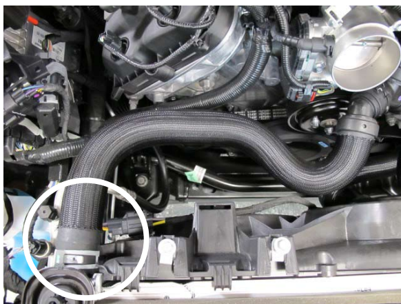
Fig. 3-i: Upper Radiator Hose (OEM Configuration)
