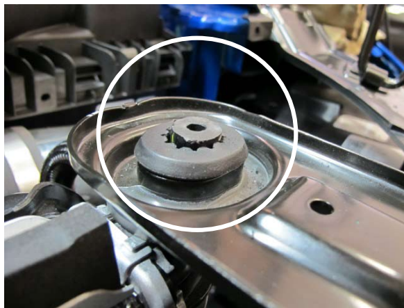
Fig. 7-n: Modify Radiator Mounting Tabs
