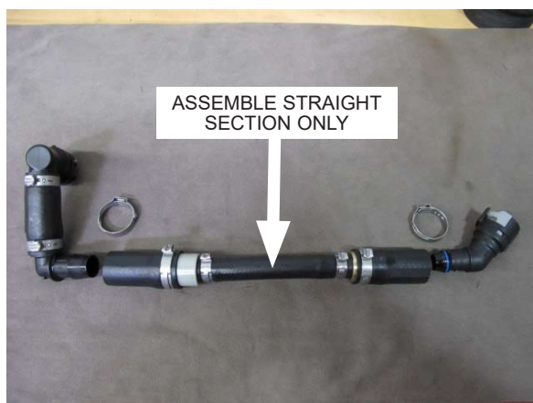
Fig. 7-c: Assemble Straight Section Of PCV Assembly
