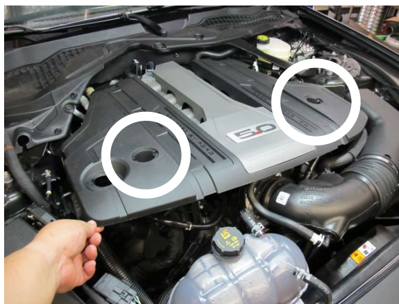
Fig. 1-t: Remove Engine Cover
