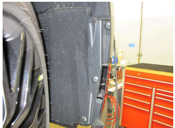
Fig. 1-f: Remove Fender Liner Fasteners
