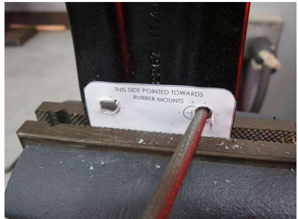
Fig. 3-d: Use Round File To Slot Hole
