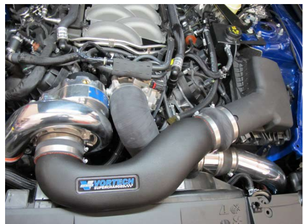
Fig. 7-l: Loosely Install Air Inlet Tube
