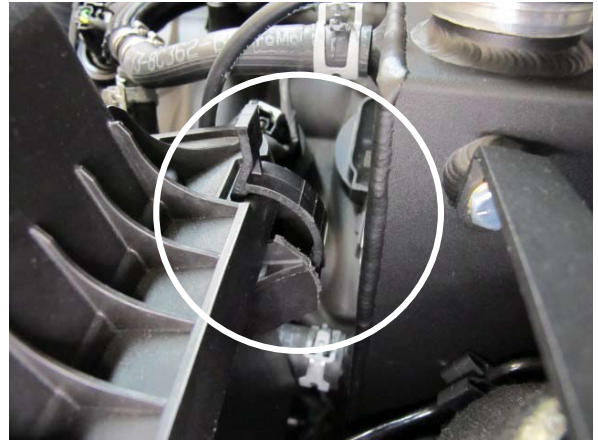
Fig. 7-g: Trim Air Box As Necessary
