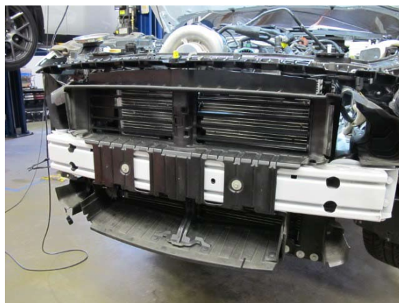
Fig. 1-o: Remove 8mm-Headed Fasteners
