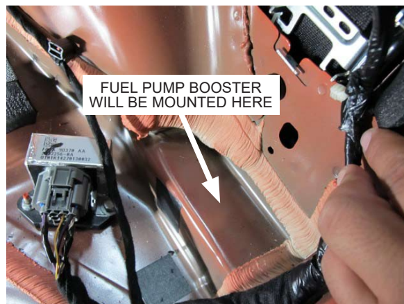
Fig. 6-j: Fuel Pump Booster Mounting Location
