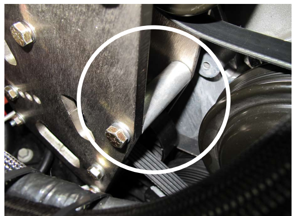
Fig. 2-r: Reinstall Previously Removed 1x 2.730" Spacer
