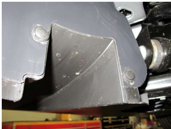
Fig. 1-g: Remove Plastic Fasteners
