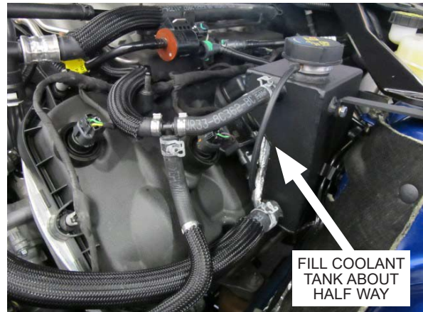
Fig. 3-y: Refill Cooling System
