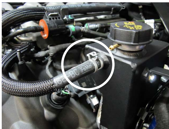
Fig. 3-t: Attach Upper OEM Molded Coolant Hose
