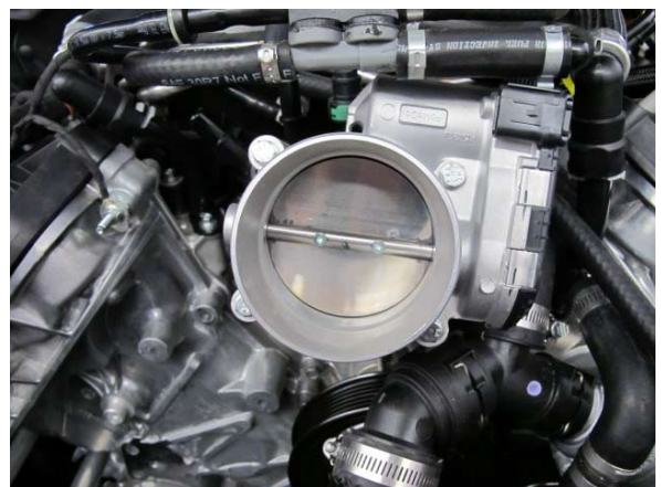
Fig. 4-c: Reinstall Throttle Body
