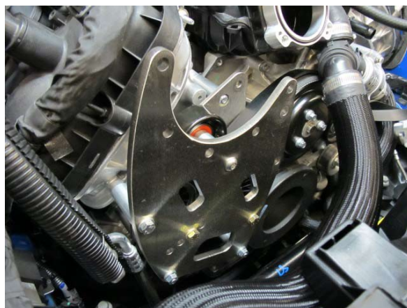
Fig. 2-i: Install Supercharger Mounting Bracket Assembly
