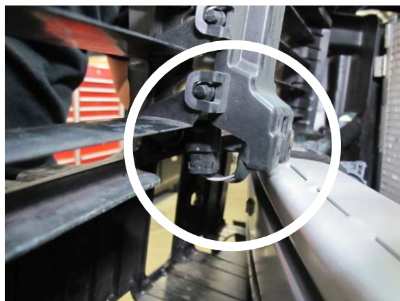
Fig. 1-s: Unplug Motor & Remove Active Grille Shutter Assembly
