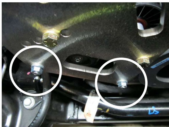
Fig. 2-l: Install 2x M8 Nuts & 2x 5/16" Washers
