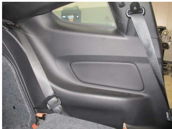
Fig. 6-g: Remove Driver Side Rear Interior Panel
