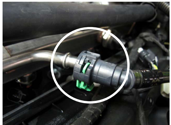
Fig. 5-f: Disconnect Low Pressure Fuel Feed Line
