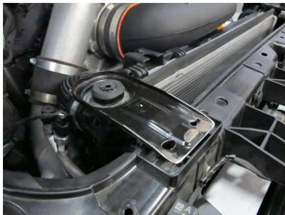
Fig. 3-g: Reinstall Modified Upper Radiator Brackets
