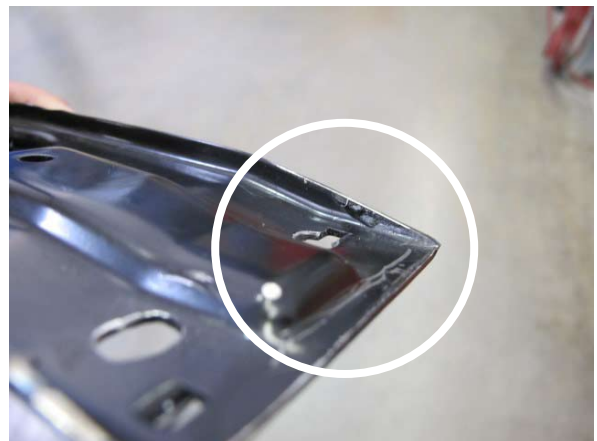
Fig. 3-f: Grind Down Raised Edges To A Taper
