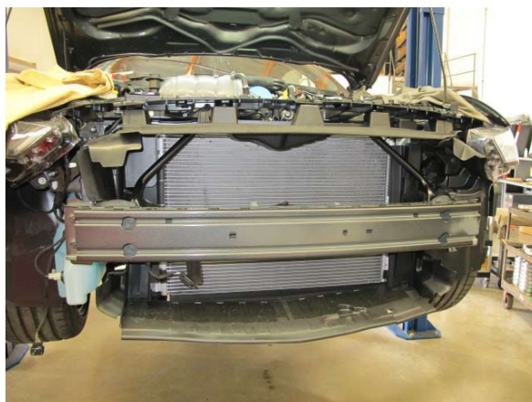
Fig. 1-m: Remove Front Bumper Cover
