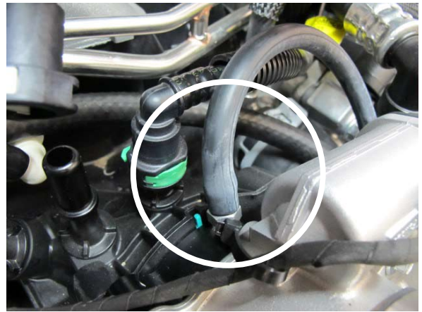
Fig. 4-ar: Attach Vacuum Hose To 1/4" Fitting
