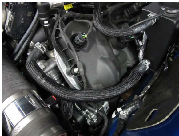
Fig. 3-w: Secure Modified OEM 3/4" Coolant Hose
