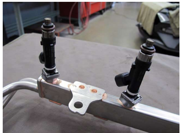
Fig. 5-i: Make Note Of Fuel Injector Orientation
