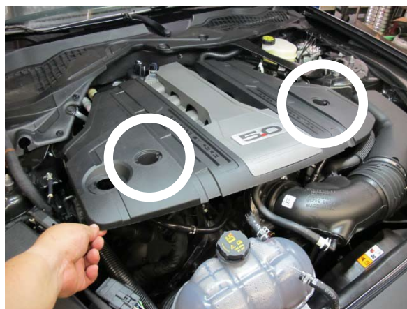
Fig. 1-t: Remove Engine Cover
