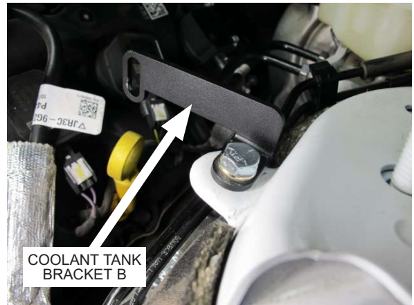
Fig. 3-q: Secure Coolant Tank Bracket B
