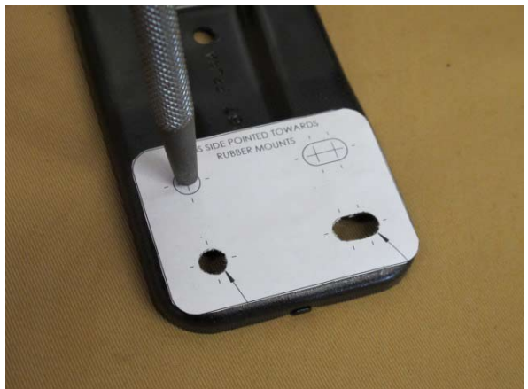
Fig. 3-c: Center Punch The Holes To Be Drilled
