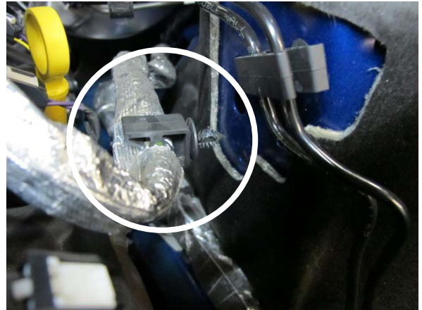
Fig. 3-p: Release EVAP Hose From Driver Side Shock Tower
