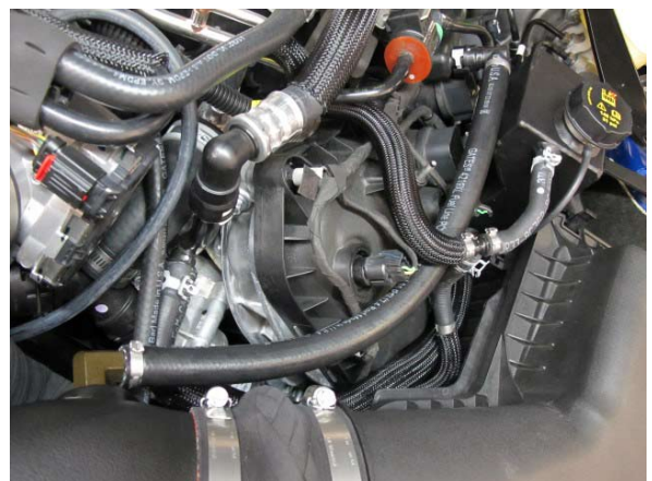
Fig. 7-i: Attach Breather Hose To Air Inlet
