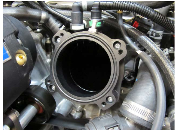
Fig. 4-b: Install Throttle Body Spacer
