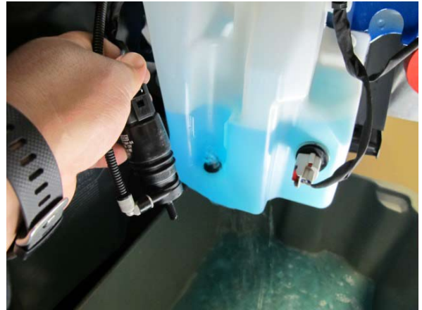
Fig. 4-d: Drain Windshield Washer Fluid Reservoir
