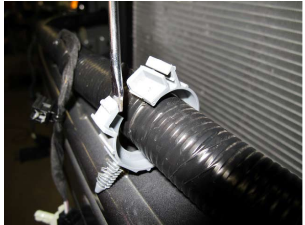
Fig. 4-p: Remove Gray Wire Harness Clips
