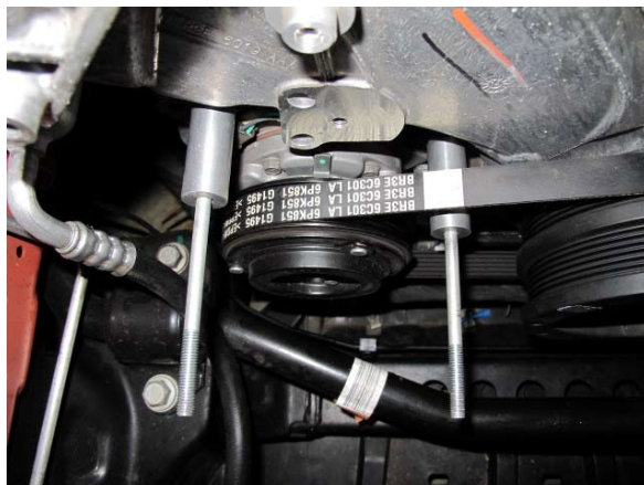
Fig. 2-g: Install 1x 2.058" & 1x 2.146" Spacers
