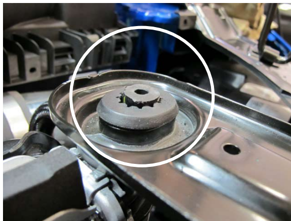
Fig. 7-n: Modify Radiator Mounting Tabs
