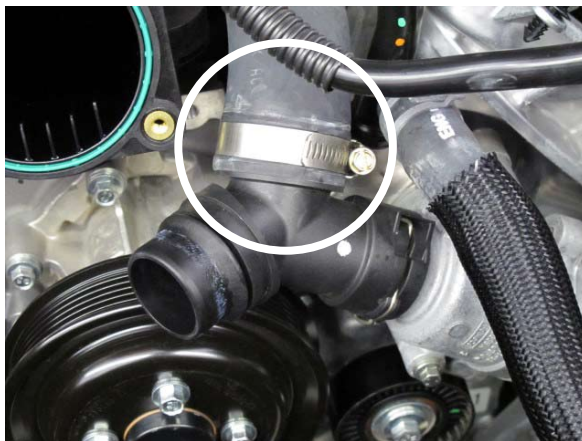
Fig. 3-h: Install #24 Hose Clamp
