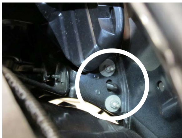
Fig. 1-i: Remove Corner Bracket Fasteners
