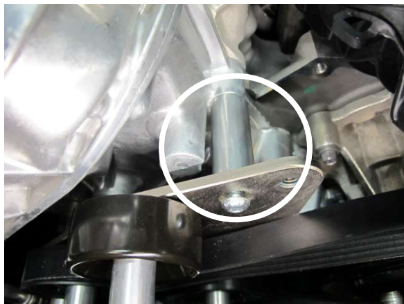
Fig. 2-j: Install 1x 2.058" Spacer
