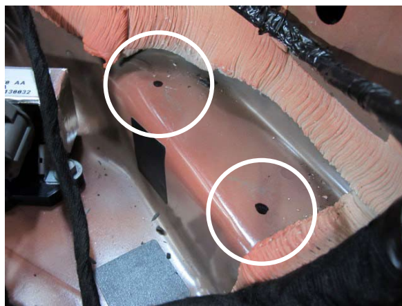
Fig. 6-k: Mark & Drill Mounting Holes
