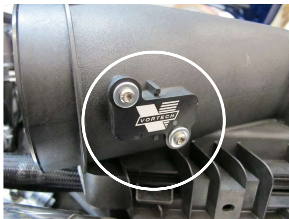
Fig. 7-f: Install MAF Block-Off Plate
