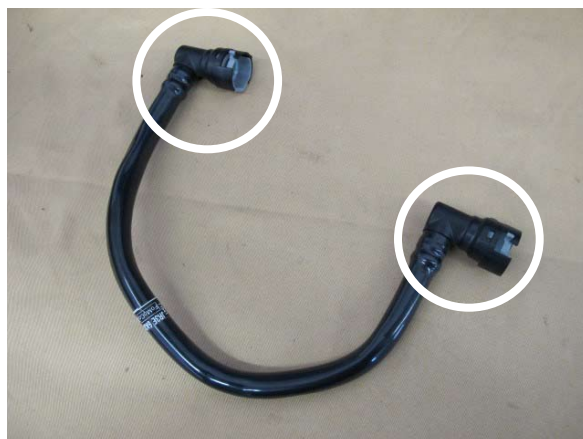
Fig. 7-a: Remove Both Quick-Release Fittings
