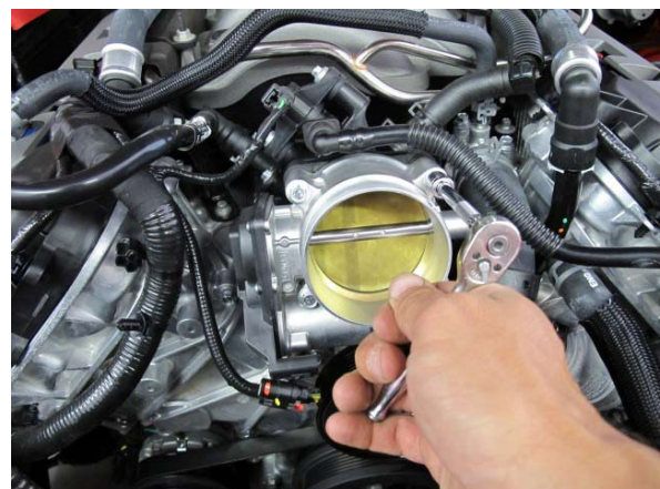
Fig. 1-aa: Remove Throttle Body
