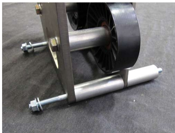
Fig. 2-h: Keep 2x 2.730" Spacers In Place
