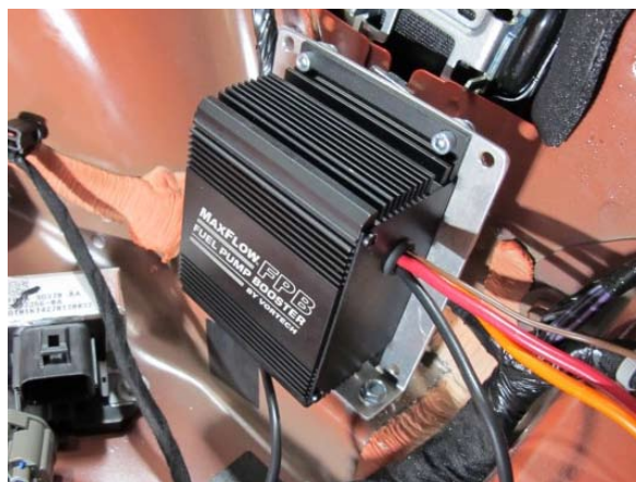
Fig. 6-l: Mount Fuel Pump Booster
