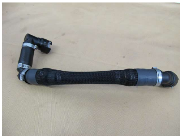
Fig. 7-d: Loosely Assemble OEM Quick-Release Fittings As Shown
