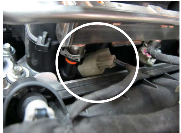
Fig. 5-d: Disconnect Fuel Injectors
