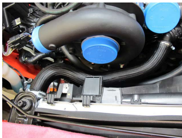
Fig. 3-k: Upper Radiator Hose (New Configuration)
