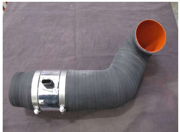
Fig. 4-ap: Assemble MAF Sensor Housing & Sleeves As Shown
