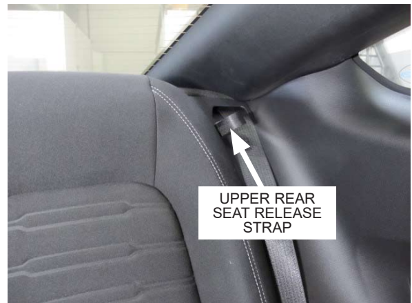
Fig. 6-d: Fold Upper Rear Seat Down
