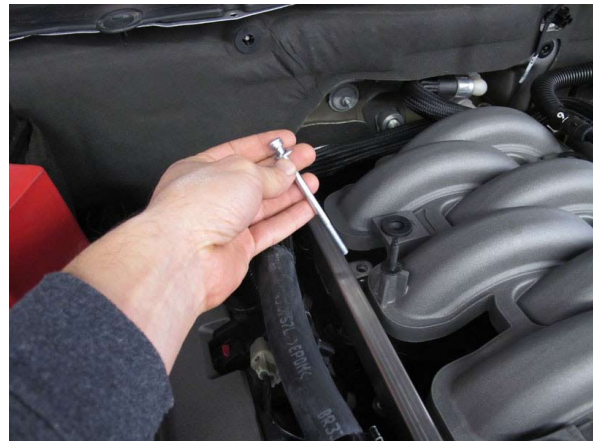
Fig. 5-h: Remove Fuel Rail Assembly
