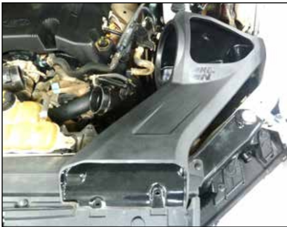
7. Install the K&N air filter housing so the mounting pin inserts into the factory grommet and then secure to the inner fender using the mounting bolt from the previous step. Install the two provided push clips into the K&N fresh air intake as shown.
