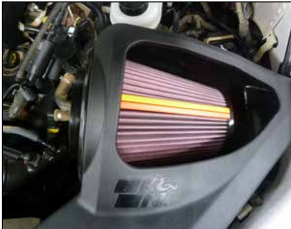
12. Install the K&N air filter into the filter housing until it locks into place.
