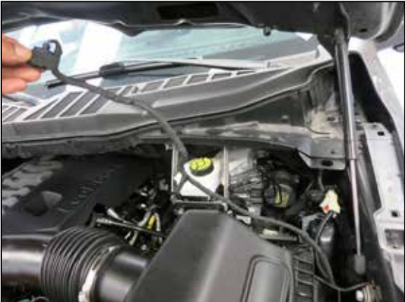
4. Disconnect the IAT sensor electrical connection and unhook the wiring harness from its mounts.
