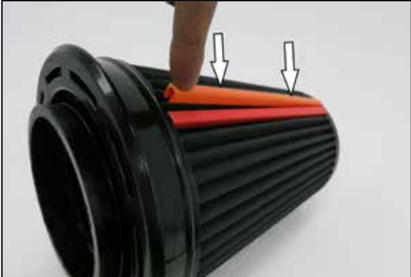
11. Attach the filter clips to the pleats on the air filter align and push down. Driver side filter, place orange clip on top and red on bottom.
