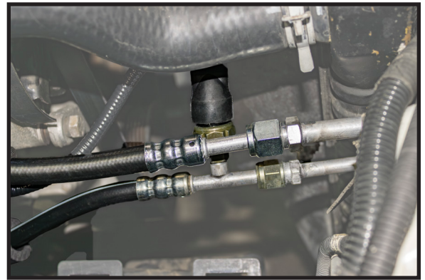
Photo 11 - Attach Pressure Safety Switch to Liquid Line Hose Assembly
