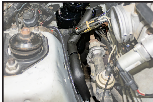
Photo 9 - Install Liquid Line Tube & use Zip Tie to secure to Shock Tower
