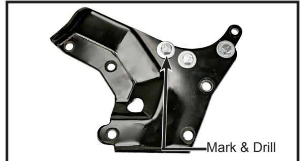
Photo 4 - Mark & drill OE Compressor Bracket to attach the Compressor Adapter Bracket
