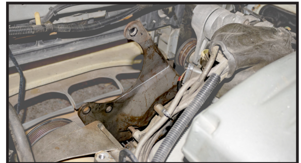
Photo 5 - Mark & trim OE Compressor Bracket
