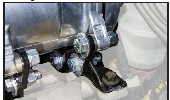
Photo 7 - Rotate & attach the Compressor Adapter Bracket to the OE Rear Compressor Bracket
