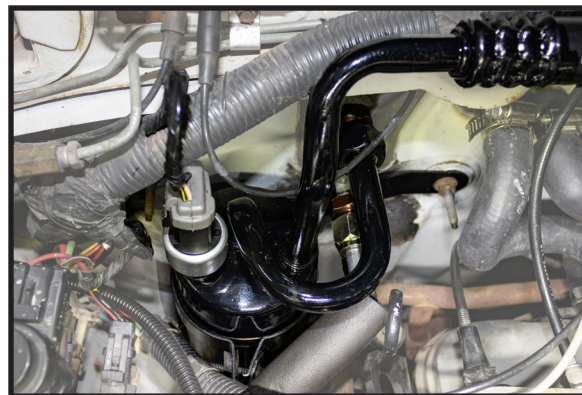
Photo 8 - Align the Accumulator to Evaporator
