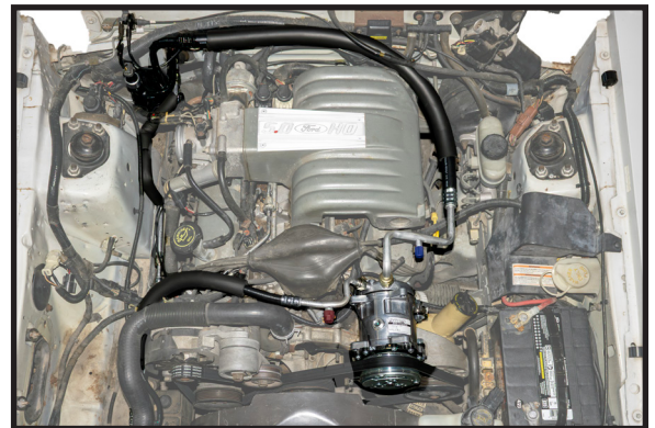
Photo 13 - Route Suction & Discharge hose from the Compressor
