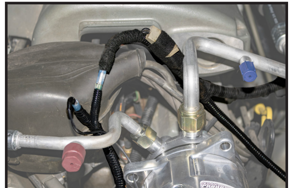
Photo 14 - Modify Factory Compressor Plug & attach to Compressor Safety Switch
