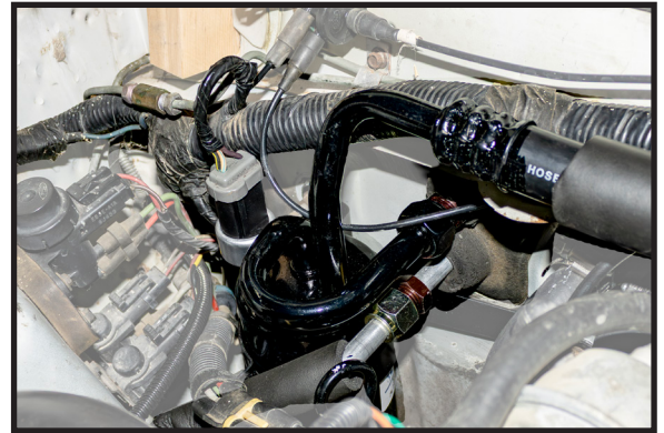
Photo 12 - Attach Pressure Cycling Switch to Accumulator
