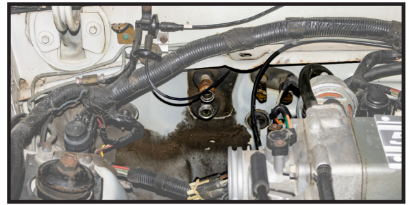
Photo 3 - Remove Accumulator & Suction Hose
