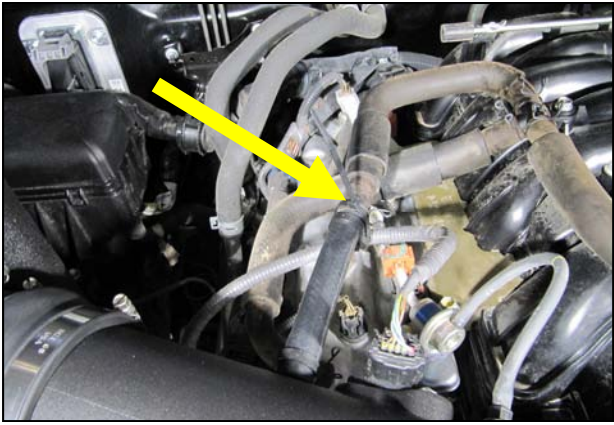
22. Use the provided Cable Tie to secure the MAF harness to the PCV line as shown. Trim excess.
