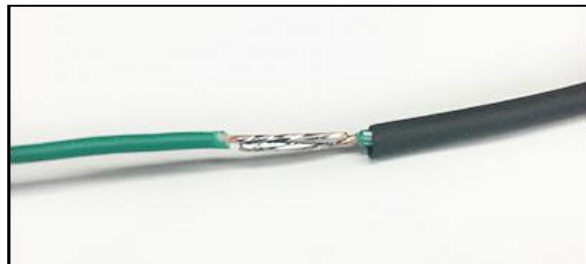
Soldered Connection w/ adhesive heat shrink
