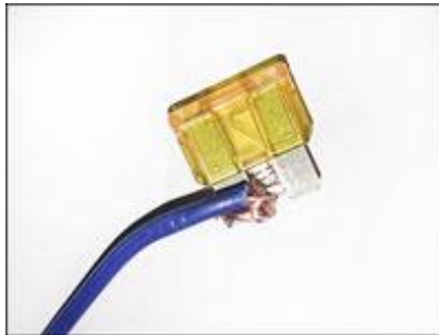
Wire Jammed Into a Fuse
