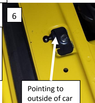
The threaded piece should be facing left to right facing the car, after inserting through hole.
