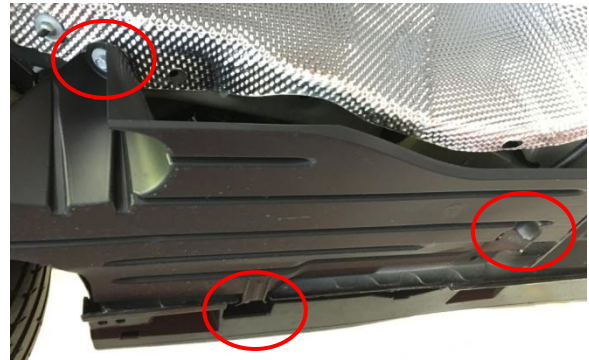
Figure 1: Rear plastic cover hardware
