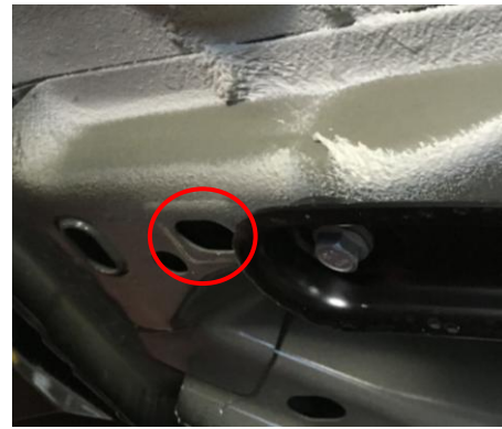
Figure 4: Slotted hole for offset stud
