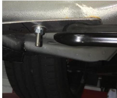
Figure 5: Steeda jacking rail front bracket
