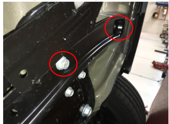
Figure 3: Cross brace bolts
