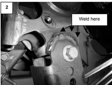
Note: The lower the position the rear mount of the control arms, the higher and shorter your instant center will be. Raising it lowers your install center and makes it longer. Not recommended for factory control arms, if used you can only use the lowest mounting hole.
