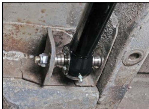
Lower links mount at OEM leaf-spring brackets.
