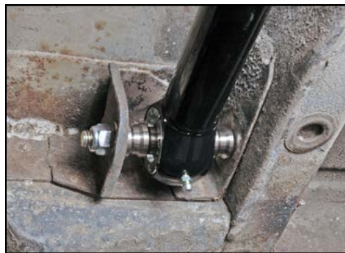
Lower links mount at OEM leaf-spring brackets.
