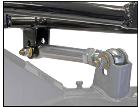
2-position chassis and housing arm brackets
