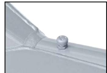
Screw-in axle vent eliminates seal damage from pressure build up.
