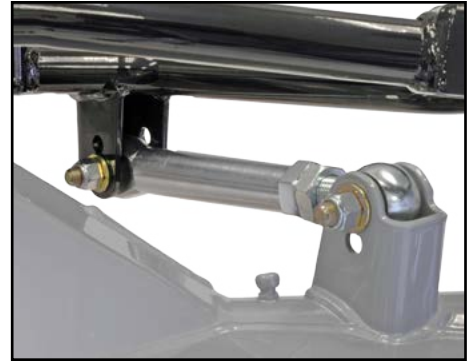
2-position chassis and housing arm brackets
