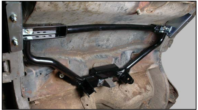
"Self-positioning" system uses existing pinion snubber and top shock mount bolt holes.
