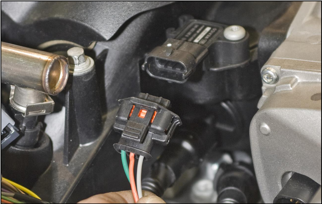
Route the m.a.p. sensor connector up to the m.a.p. sensor, which is located front and center top of the intake manifold. Plug it in as shown here.
