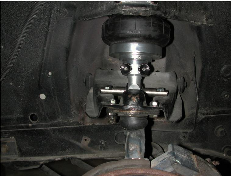
3. Hold the upper Shockwave mount up to the bottom of the strut tower. Place the upper aluminum plate on top of the strut tower. These two mounts will sandwich the strut tower using the three 5/16" x 1" Flange bolts supplied. You may have to drill them out.
