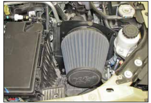
17. Install the K&N® air filter onto the filter adapter and secure with the provided hose clamp.
