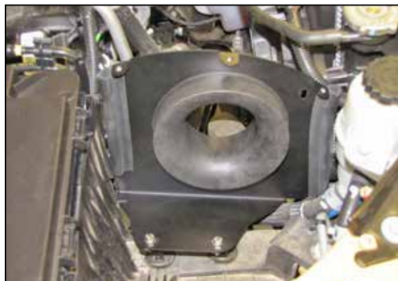
16. Install the heat shield assembly into position so the mounting studs are in the air box mounting grommets.
