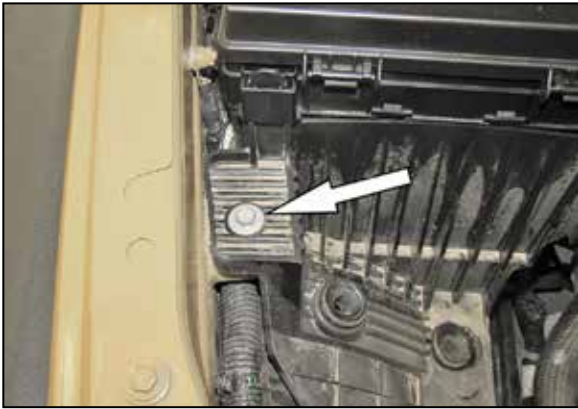
9. Remove the bolt show that secures the air box mount bracket to the inner fender.
