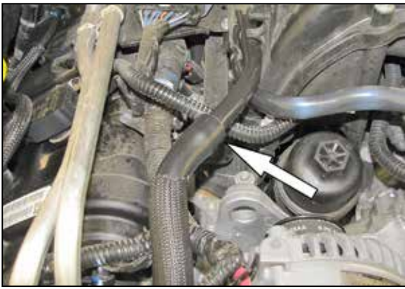
7. Disconnect the crank case vent hose from the crank case vent tube.
