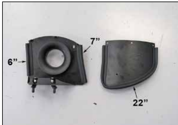
15. Install the edge trim onto the heat shield and lid as shown.
