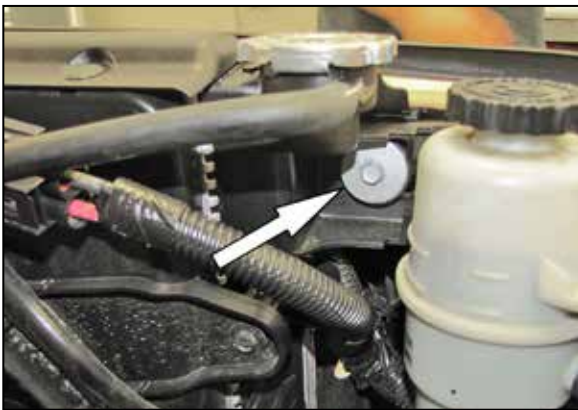
10. Remove the bolt show that secures the radiator to the core support.
