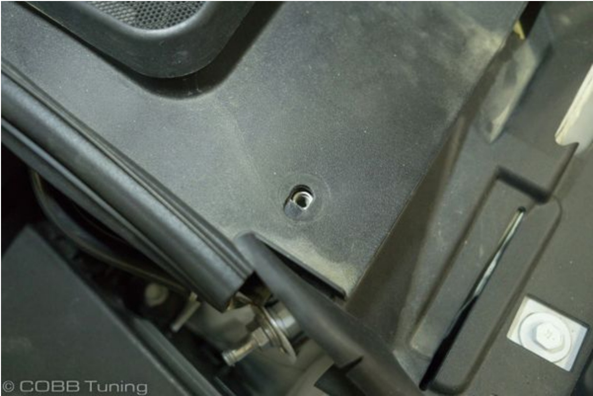
3. Remove (4) pressure clips securing the front windshield cowl using a flathead screwdriver.
