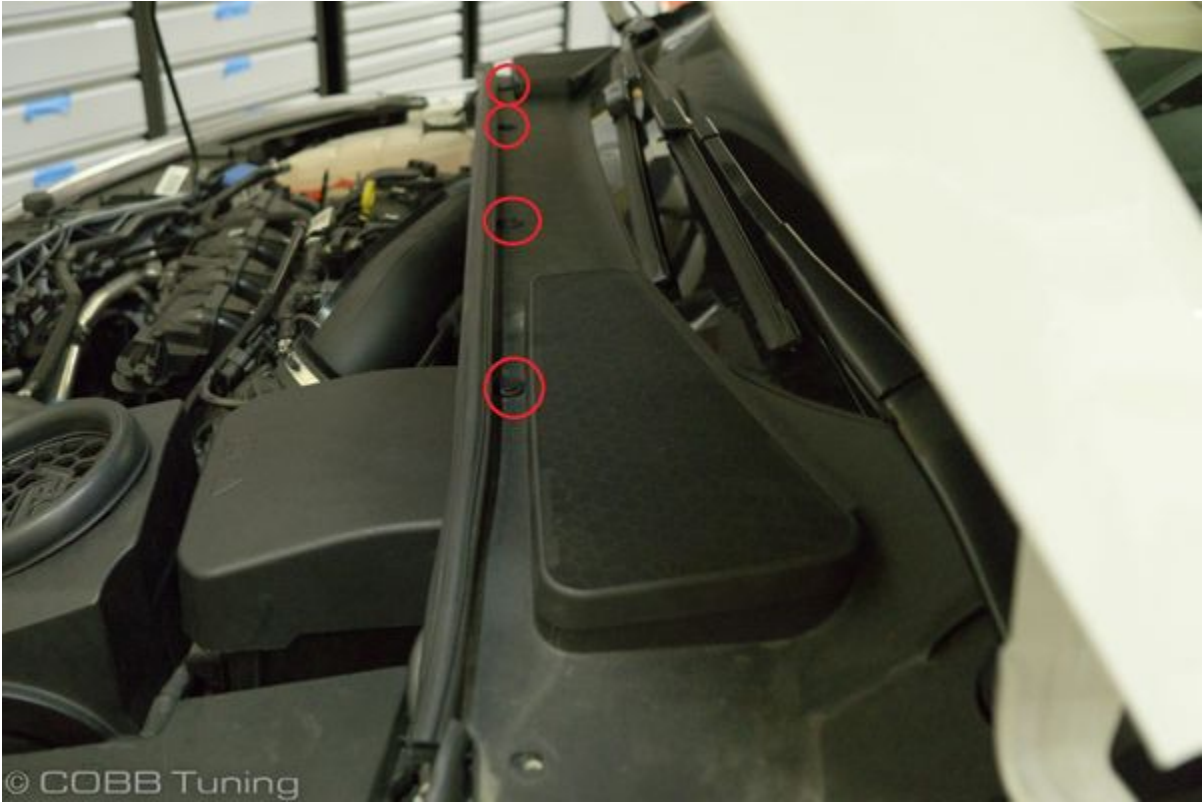
3. Remove (4) pressure clips securing the front windshield cowl using a flathead screwdriver.
