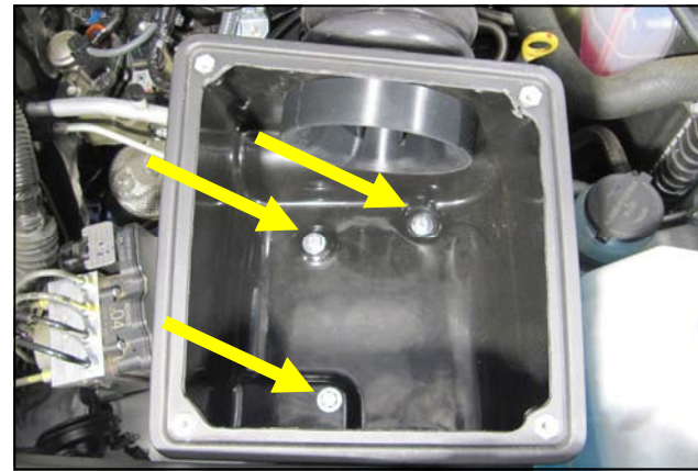
17. Mount the Airaid Airbox onto the CAB Mounts using the three 8mm Bolts and 5/16 Flat Washers
