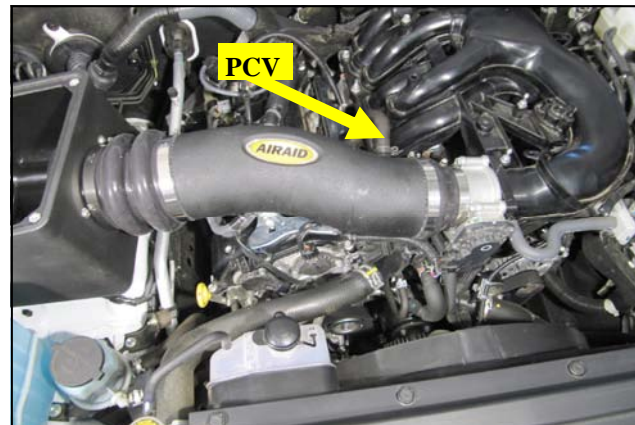
14. Insert the Intake tube into the Hump Hose and coupler. Align the tube with the PCV line, re connect it and tighten all 4 Clamps.
