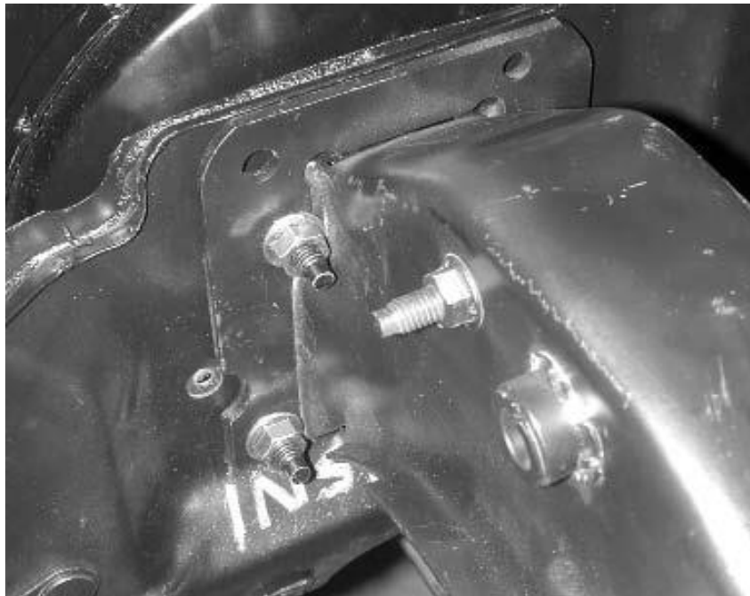
Figure 3 – Mounting the Brake Booster and Pedal Box
