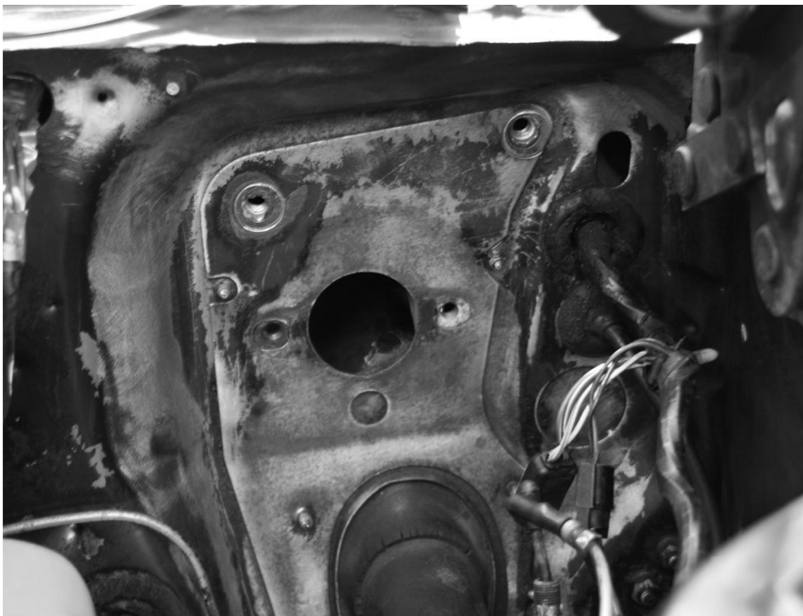
Figure 1 – Firewall Ready to Start Installation
