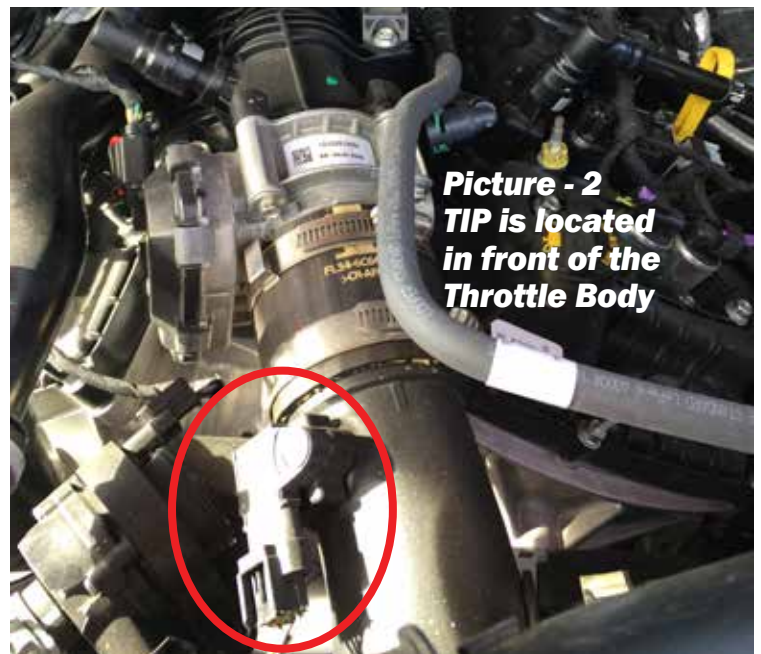
Picture - 1 TIP is located in front of the Throttle Body on the inlet 2.7L EcoBoost
