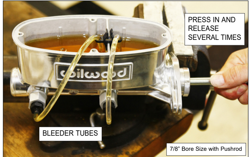
Typical Bleeder Tube Setup and Use
