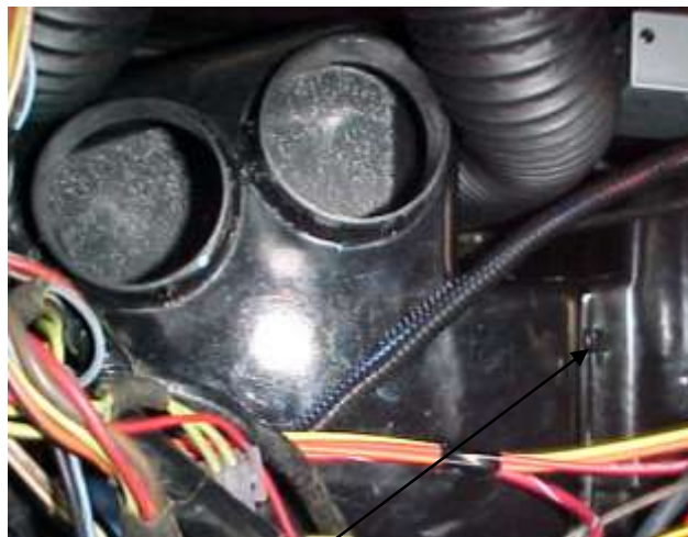
#10 x 5/8" pan head philips screw
